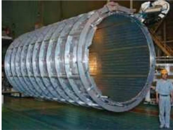
Figure 2.16: The ATLAS central Solenoid
