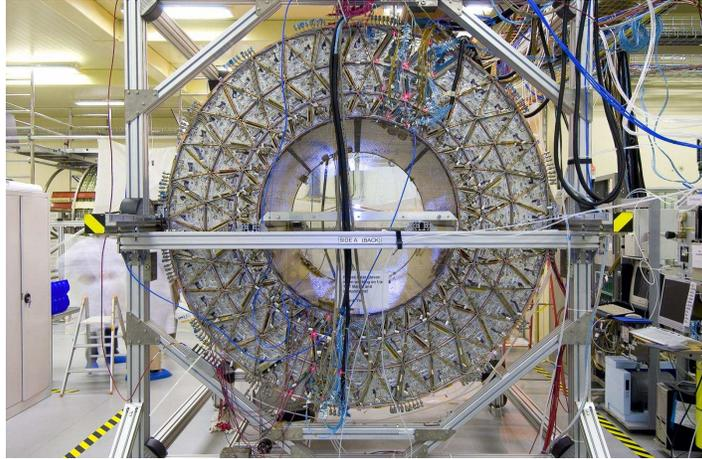
994 of straws per track guarantees a measurement accuracy of better than  $50\ \mu\text{m}$  averaged
