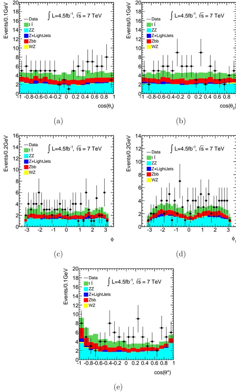
Figure 5.20: Angular distributions for the  $4\mu$  and  $2e2\mu$  reference OS CR events at  $\sqrt{s} = 8$  TeV: (a)  $\theta_1$ , (b)  $\theta_2$ , (c)  $\phi$ , (d)  $\phi_1$  and (e)  $\theta^*$ . The reducible background is normalized to the estimations made using the nominal fit, the irreducible background is taken from the MC and no signal MC is included.
