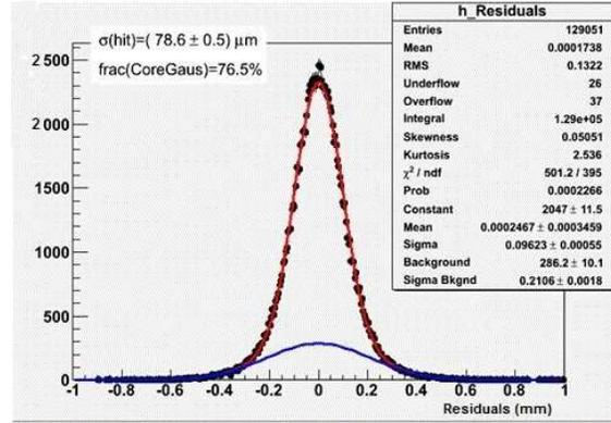
2549 resolution is estimated by fitting the residuals distribution, shown in Figure 4.32, with a
