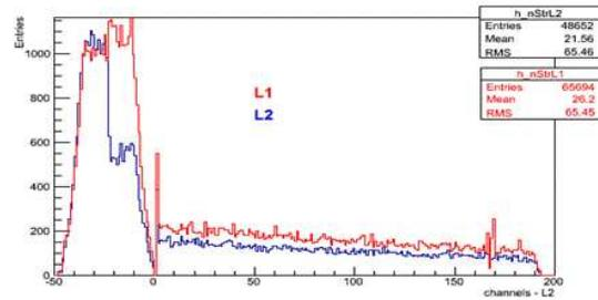
Figure 4.46:  $C05L1$  less occupancy associated with the lower current drawn in the middle of the data taking (June 13<sup>th</sup>, 2012). The source is probably due to a failure in the HV distribution line. The image is a screen shot from the DCS viewer.
