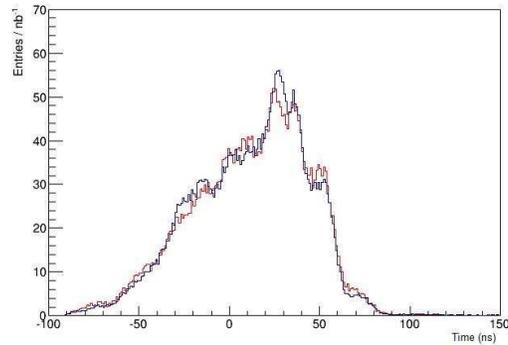
Figure 4.53: The unspoiled hits on segments for 25 ns (red line) and 50 ns (blue line) data. Due to the smaller contamination with small amplitude hits, the unspoiled fraction is higher for the 25 ns data.
