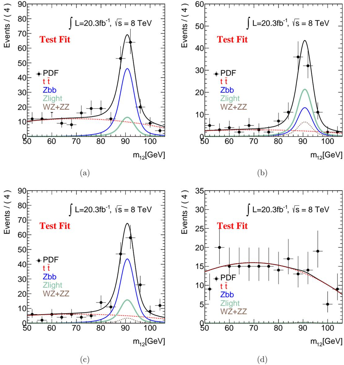
Figure C.4: The data  $m_{12}$  distributions are presented after the test fit, where the  $Zb\bar{b}$  and  $Zlight$  are treated as one background, the  $Zjets$ , for testing reasons. The CRs of the inverted  $d_0/\sigma d_0$  (a), inverted isolation and nominal  $d_0/\sigma d_0$  (b), SS (c) and  $e\mu + \mu\mu$  (d) are presented. The test proves no significant deviation with the nominal results.
