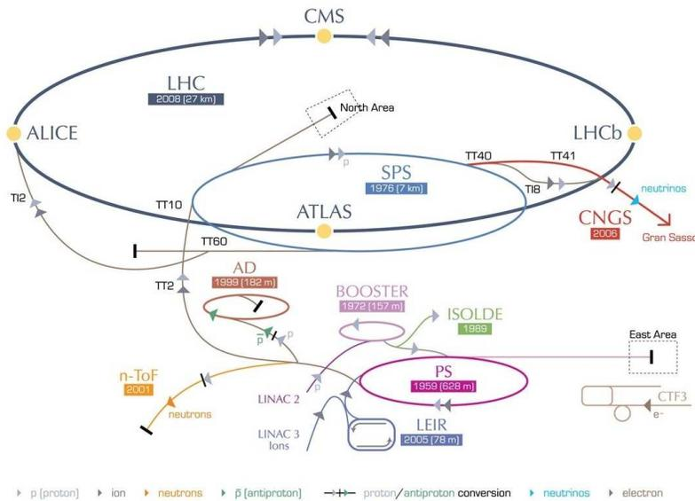
spacing. During the Run-I period the bunch spacing was 50 *ns* and it is expected to be half during the Run-II operation. The SPS is the final step before the beam transferred to the LHC with an energy of 450 GeV both in clockwise and counter-clockwise directions after a filling time of 4.20 *minutes* per LHC ring. In the LHC, the beams circulate until they ramp to high energy and can be stored up to 10 *hours*, this is the so called "beam lifetime".
