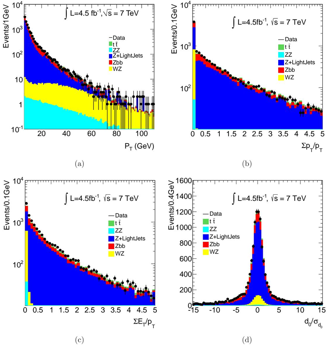
Figure 5.6: Properties of the muons accompanying a  $Z$  candidate before the application of the isolation and impact parameter selection using the 2012 data: (a)  $p_T$  spectrum, (b) normalized track-based isolation, (c) normalized calorimeter-based isolation and (d)  $d_0/\sigma_{d_0}$ .
