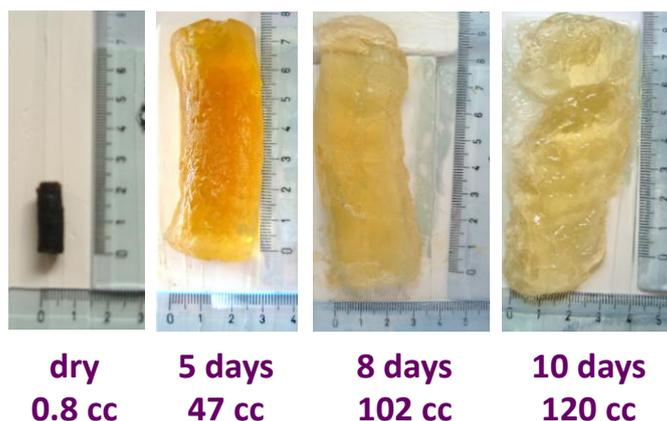
Figure 40: Swelling of a  $W_2$ -PDCPD gel in toluene.
