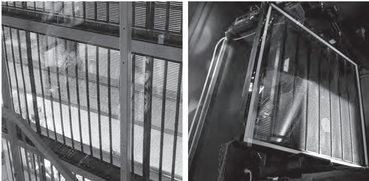
Figure 68: New transparent solar thermal collector. The left-hand photo demonstrates the possibility of visual contact from indoors to outdoors. The photo on the right-hand side shows the new facade element mounted in the Testlab Solar Facades at Fraunhofer ISE in Freiburg, Germany. Pictures © ZAG, Ljubljana, Slovenia and Fraunhofer ISE, Freiburg, Germany.
