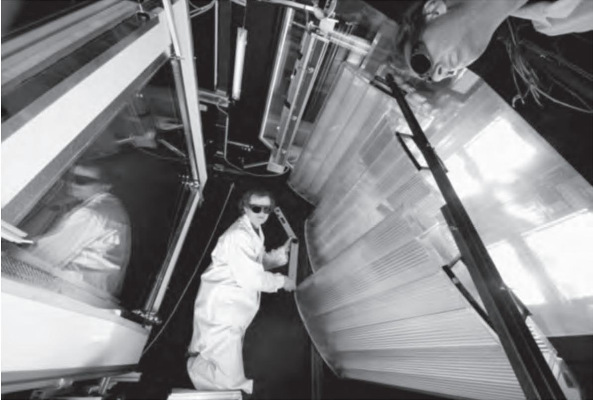
Figure 65: External blind consisting of large-scale slats, each with an ellipsoidal cover mounted for measurement in the calorimeter in the TestLab Solar Facades at the Fraunhofer Institute for Solar Energy Systems ISE in Freiburg, Germany. The slats have integrated translucent and opaque sections in order to enhance the daylighting and glare protection functionality. Pictures ©Fraunhofer ISE.
