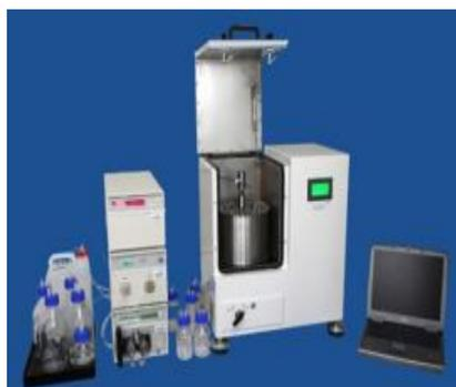
Figure 25. PLE apparatus (ASE 300, Dionex) in University of Athens, Laboratory of Pharmacogony
