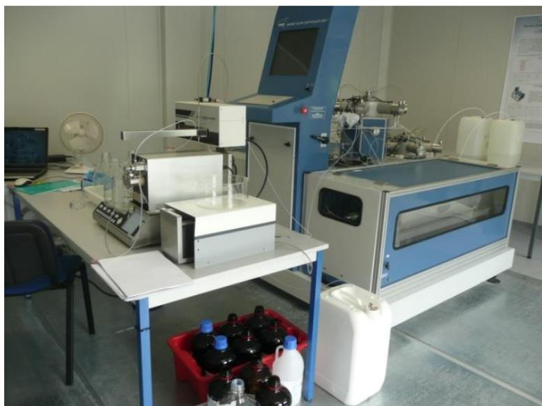
Figure 63. CCC with pilot column (Armen®, 2x6,25 lt) in ARMEN SA, Vannes, France
