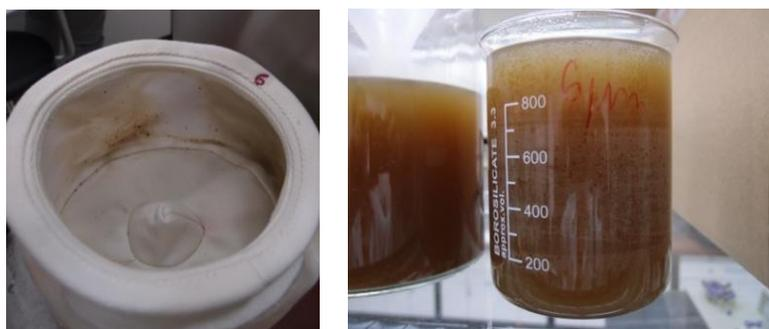
Figure 58. 6 $\mu\text{m}$  filtration bag after TOPW filtration and TOPW after filtration
