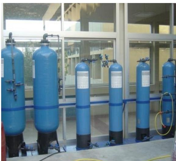
Figure 38. Pilot-scale macroporous resin columns (125 and 250 lt) in University of Athens, laboratory of Pharmacognosy
