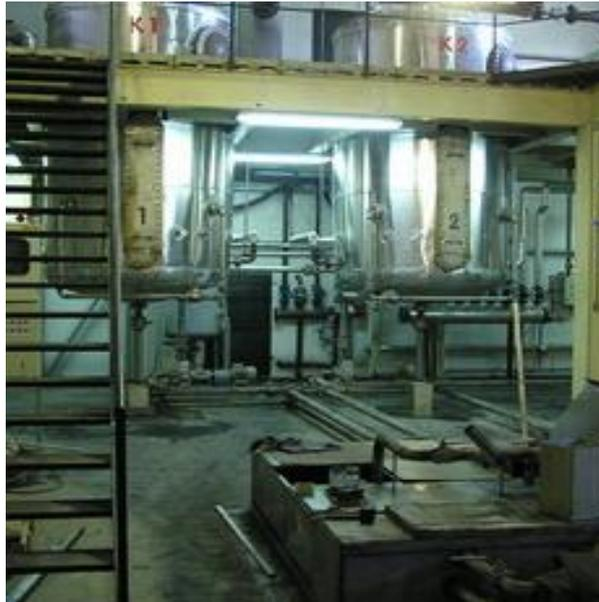
Figure 12. Tanks for the storage of deodorized oil
