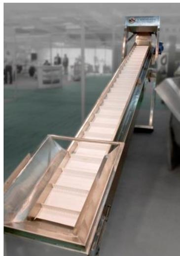
Figure 4. Defoliation equipment in a modern olive mill
