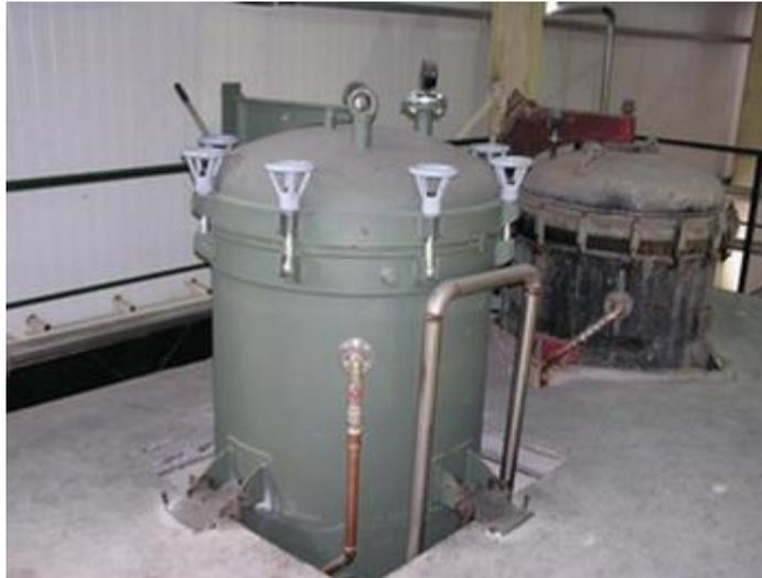
Figure 11. Oil separation filter and bleaching earth
