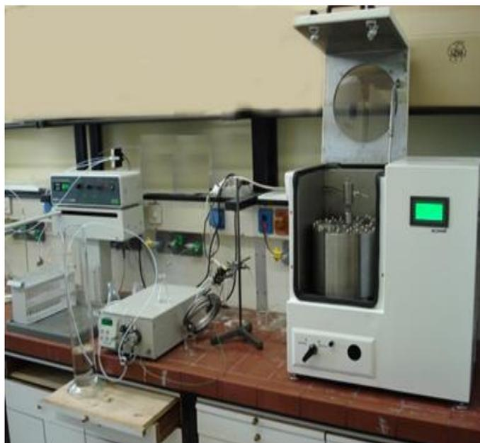
Figure 41. CCC with preparative column (Kromaton FCPC®, 1 lt) in University of Athens, laboratory of Pharmacognosy
