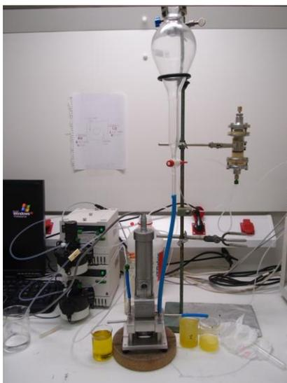
Figure 59. BXP012 liquid/liquid countercurrent extractor
