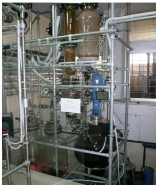
Figure 39. Pilot-scale solvent evaporation unit under vacuum (200 lt, QVF), University of Athens, laboratory of Pharmacognosy
