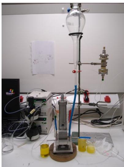
Figure 40. Rousselet-Robatel BXP012 liquid/liquid extractor
