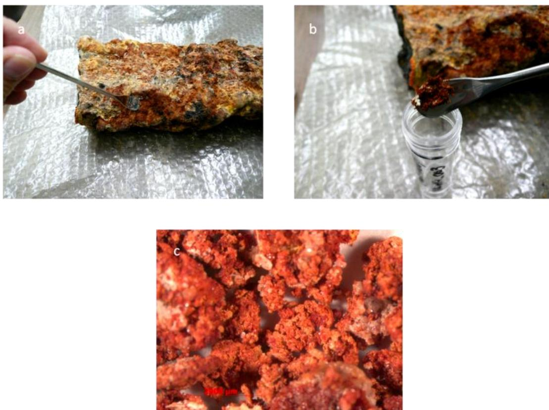
Fig.5.9 (a) Orange-yellow outer As-sulphide-dominated layer (OASL) of Politeia spire 1, (b) small pieces recovered by OASL (c) detail of b in reflected microscope.
