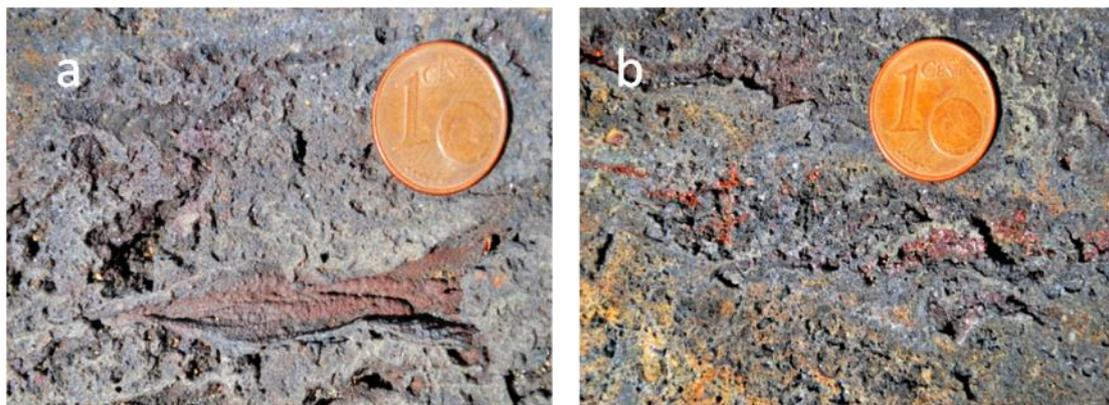
Fig.5.8 Unidentified dark-violet phases similar to Sb-Zn-S are lining interior porous conduit network of (a) Sample NA014-003 (IPCN) –in polished thin section FG3( Fig.2.5) (b) Sample NA014-003 (IPCN) –polished thin section EFG5'(Fig.2.5).
