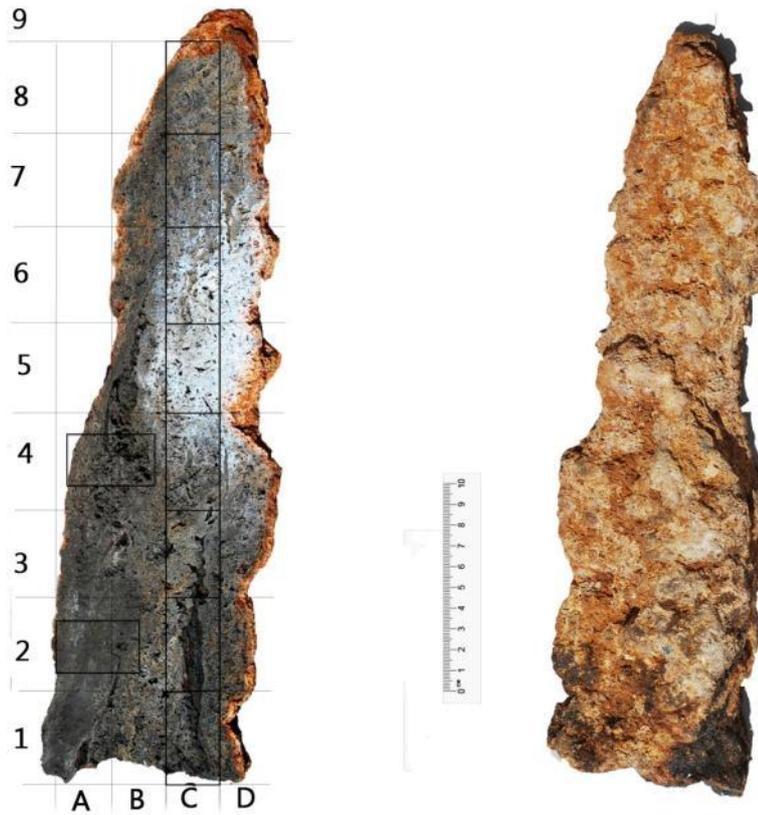
Fig.5.6 (a) Interior cut face of one half of NA014-039. Polished thin sections (C2, C3, C4, C5, C6, C7, AB2', AB4') were made based on a grid sampling strategy explained in the text. (b) View of exterior surface.
