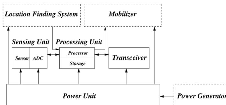
Figure 1: The components of a sensor node.
