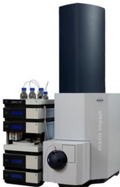
**Fig.15:** *The UHPLC-QToF-MS system*
