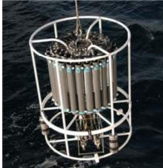
*Fig. 1.3 A CTD rosette is lowered into the water to measure the salinity, temperature, depth and concentration of particles in the water column (courtesy of NOAA Okeanos Explorer Programm, INDEX-SATAL 2010).*
