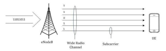
Graphic 1.14: This graphic illustrates how the incoming data is separated and transferred across different subcarriers through the OFDMA technique.
