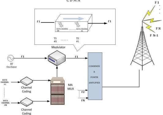
Graphic 1.6: This graphic illustrates how several transmitters can send information simultaneously over a single communication channel.
