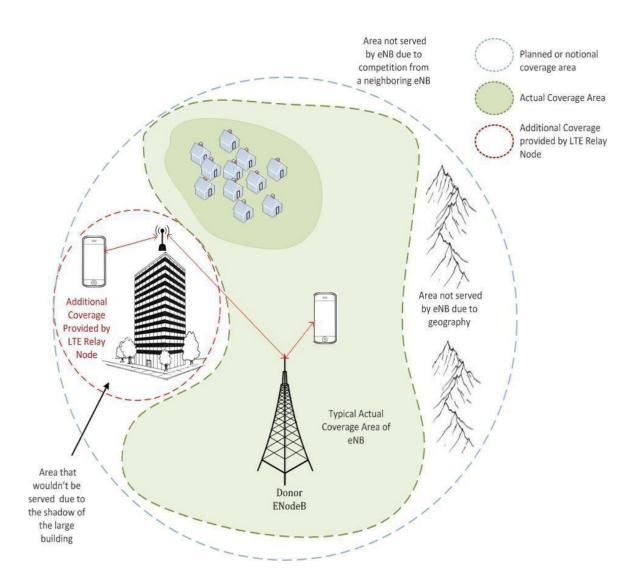
Graphic 1.18: This graphic illustrates how actual coverage is increased by the use of an LTE Relay Node.
