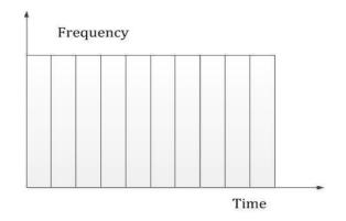
Graphic 1.4: This figure illustrates how TDMA would allocate a timeslot to a particular subscriber in a 2G wireless system.
