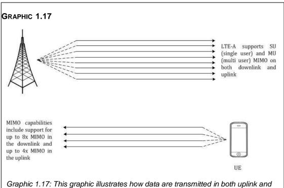
Graphic 1.17: This graphic illustrates how data are transmitted in both uplink downlink, through MIMO technique.
