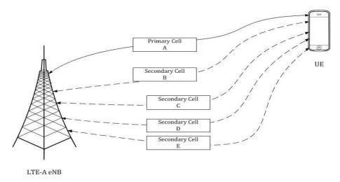
Graphic 1.19: This graphic illustrates how an eNodeB can assign capacity to a UE on multiple cells simultaneously.
