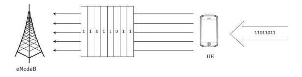
Graphic 1.15: This graphic illustrates how the incoming data is separated and transferred across different subcarriers through the SC-FDMA technique.
