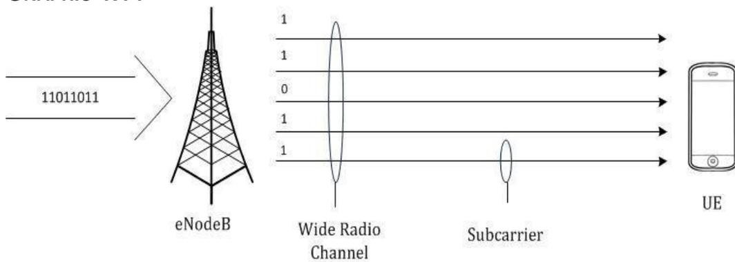
*Graphic 1.14: This graphic illustrates how the incoming data is separated and transferred across different subcarriers through the OFDMA technique.*
