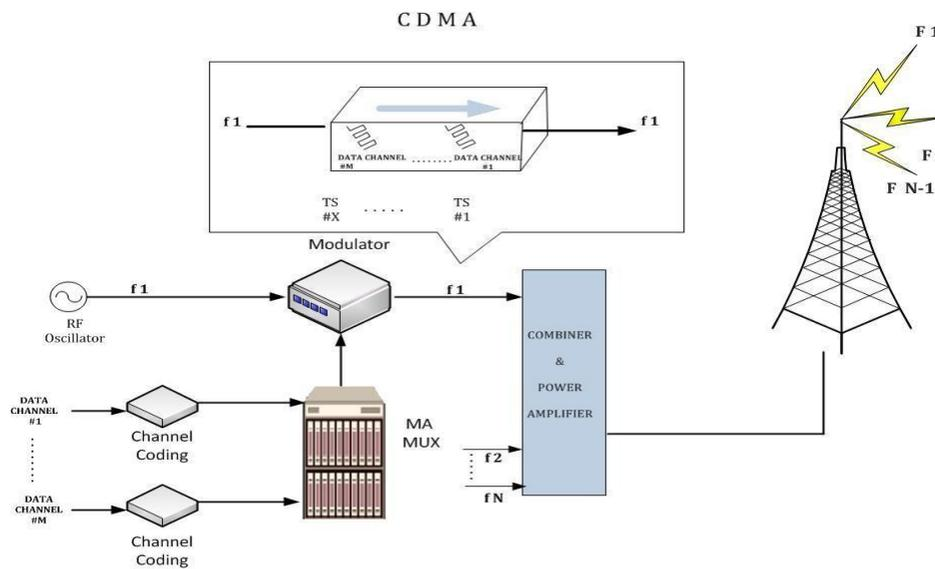
*Graphic 1.6: This graphic illustrates how several transmitters can send information simultaneously over a single communication channel.*
