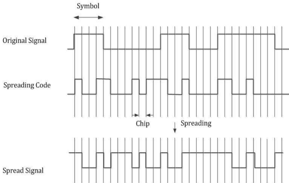
*Graphic 1.11: This graphic illustrates how the incoming signal is transformed and spread through W-CDMA technique.*
