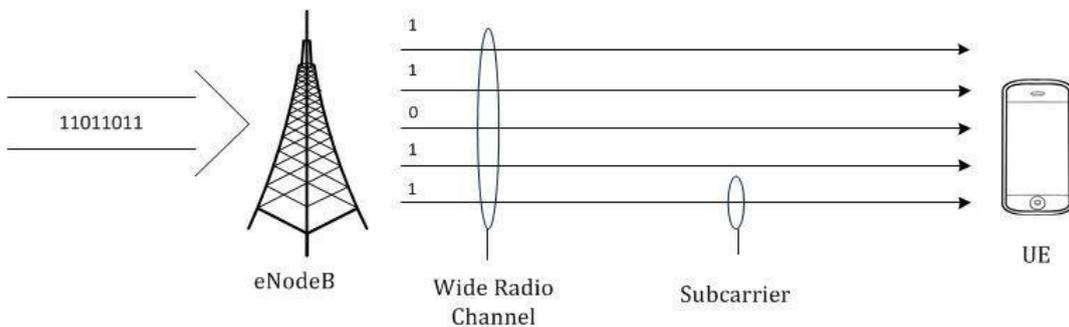
Graphic 1.14: This graphic illustrates how the incoming data is separated and transferred across different subcarriers through the OFDMA technique.
