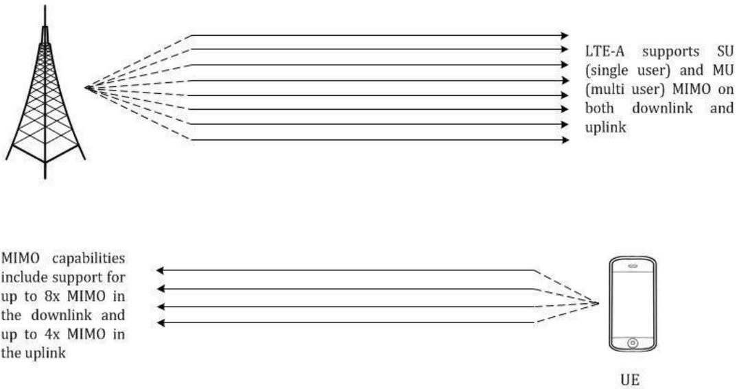
*Graphic 1.17: This graphic illustrates how data are transmitted in both uplink and downlink, through MIMO technique.*
