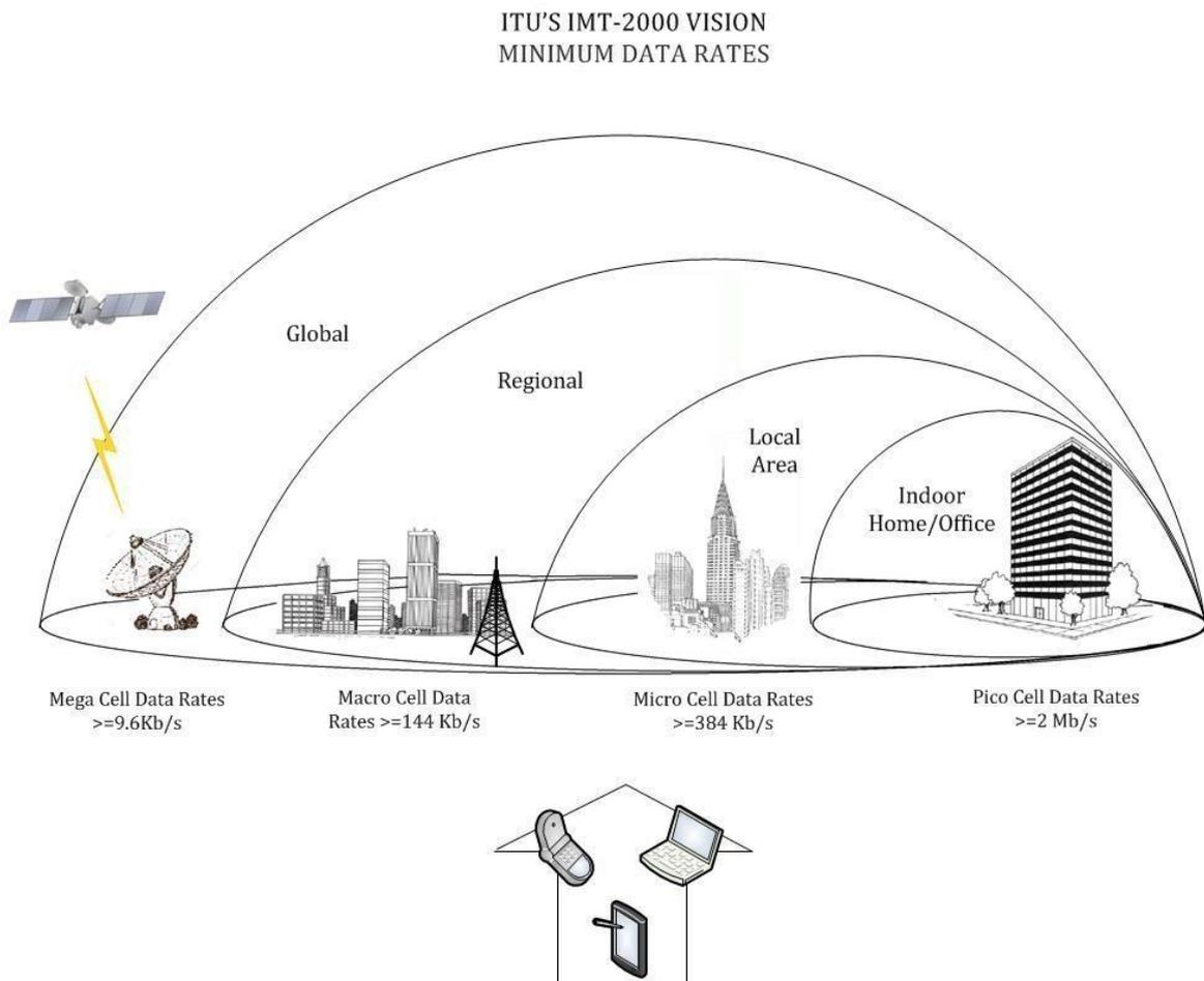
*Graphic 1.10: This graphic illustrates the ITU'S vision for the minimum data rates that third generation systems should support.*
