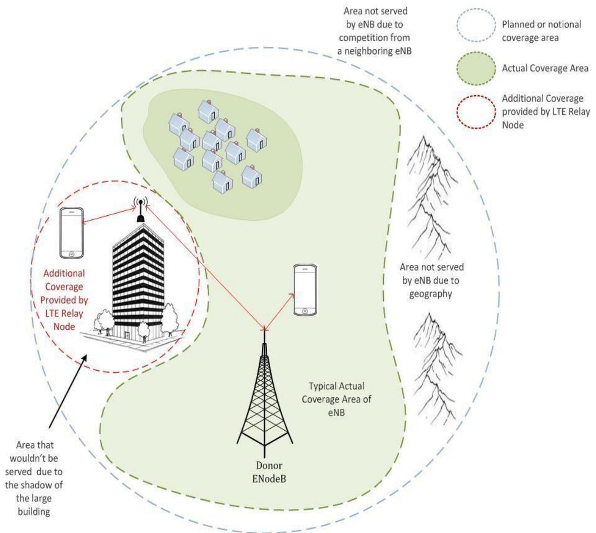
Graphic 1.18: This graphic illustrates how actual coverage is increased by the use of an LTE Relay Node.
