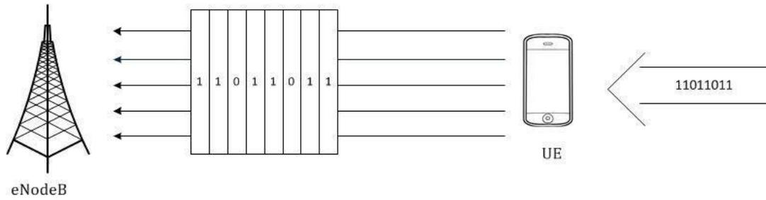
*Graphic 1.15: This graphic illustrates how the incoming data is separated and transferred across different subcarrier through the SC-FDMA technique.*
