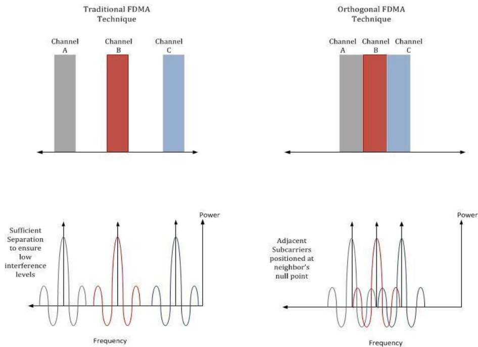
*Graphic 1.13: This graphic illustrates the difference between the traditional and the orthogonal FDMA technique*
