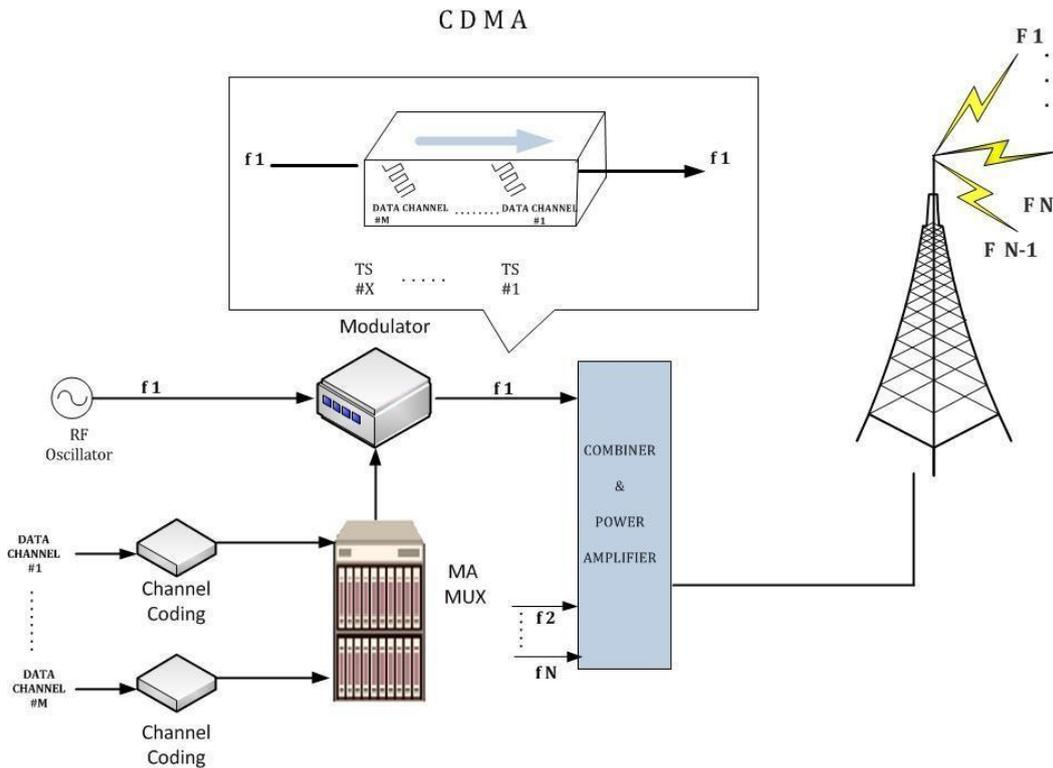
Graphic 1.6: This graphic illustrates how several transmitters can send information simultaneously over a single communication channel.
