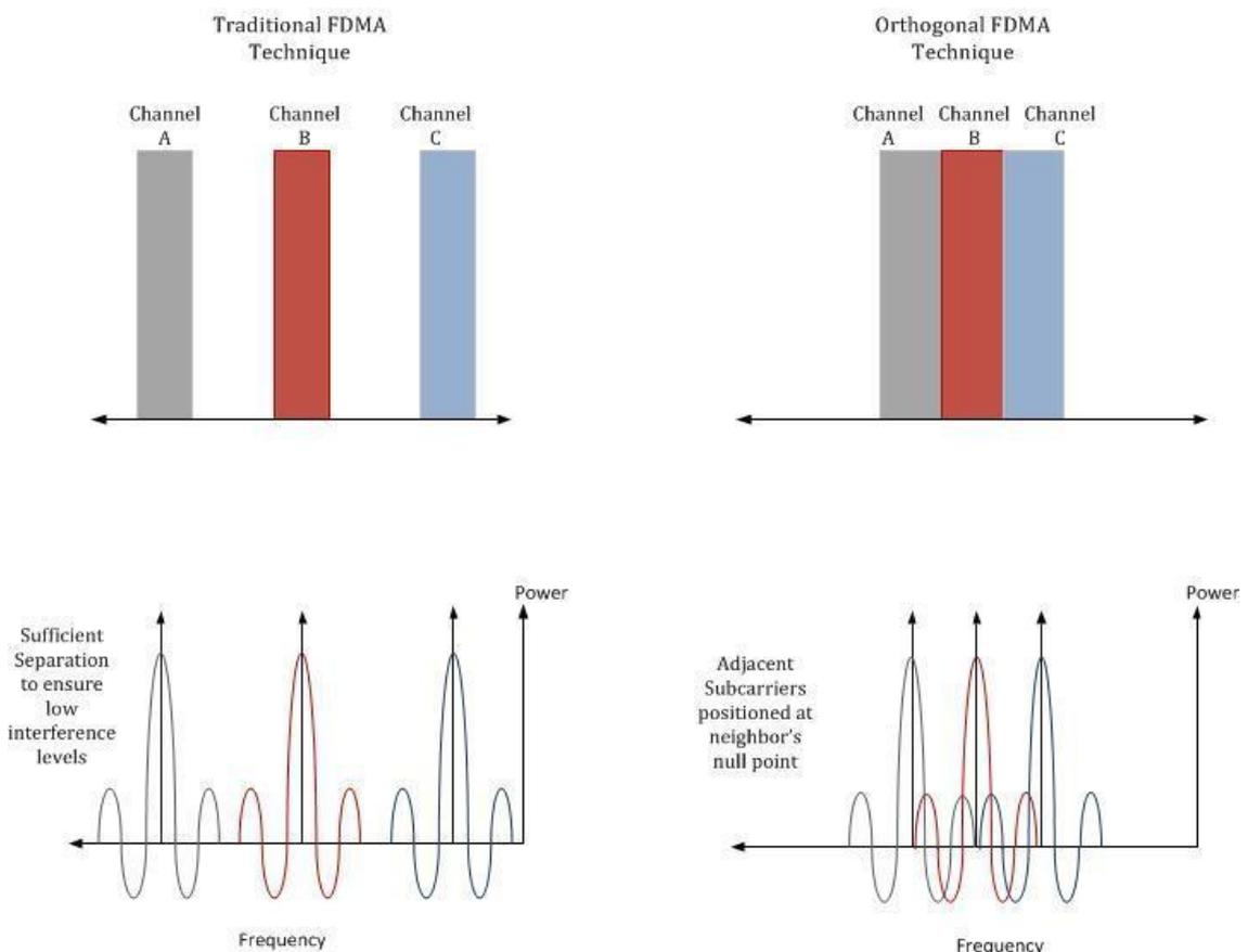
Graphic 1.13: This graphic illustrates the difference between the traditional and the orthogonal FDMA technique
