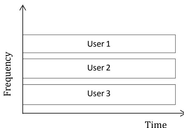
*Graphic 1.2: This graphic illustrates how FDMA would allocate a subcarrier to a particular user in a 1G wireless system.*
