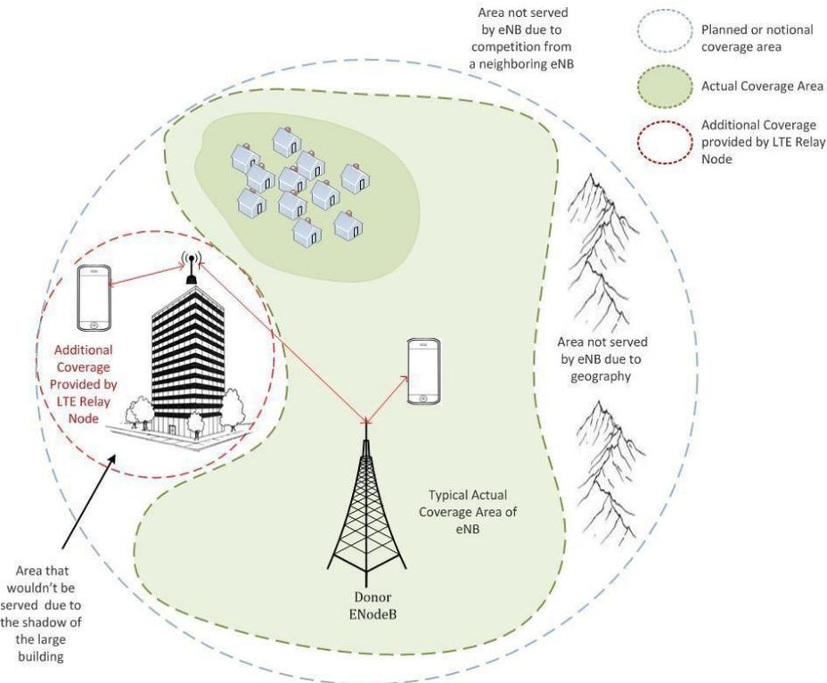
*Graphic 1.18: This graphic illustrates how actual coverage is increased by the use of an LTE Relay Node.*
