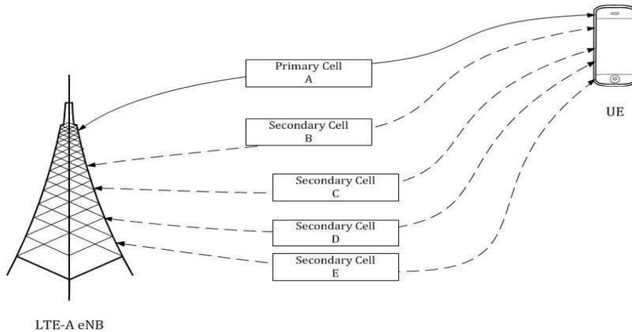
*Graphic 1.19: This graphic illustrates how an eNodeB can assign capacity to a UE on multiple cells simultaneously.*
