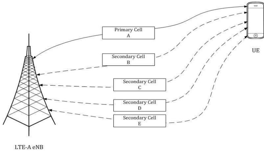
*Graphic 1.19: This graphic illustrates how an eNodeB can assign capacity to a UE on multiple cells simultaneously.*
