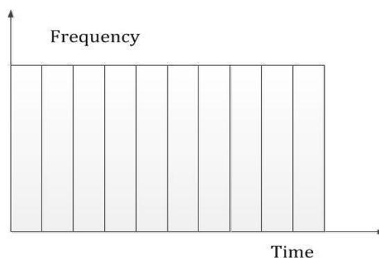
*Graphic 1.4: This figure illustrates how TDMA would allocate a timeslot to a particular subscriber in a 2G wireless system.*
