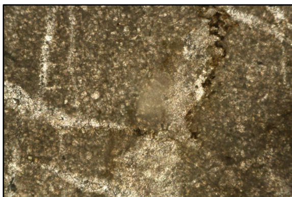
Figure 79: Section D, Senonian limestone, Sample A 2 1: Bioclastic limestone (Folk) – Packstone (Dunham), High Energy (HE).
