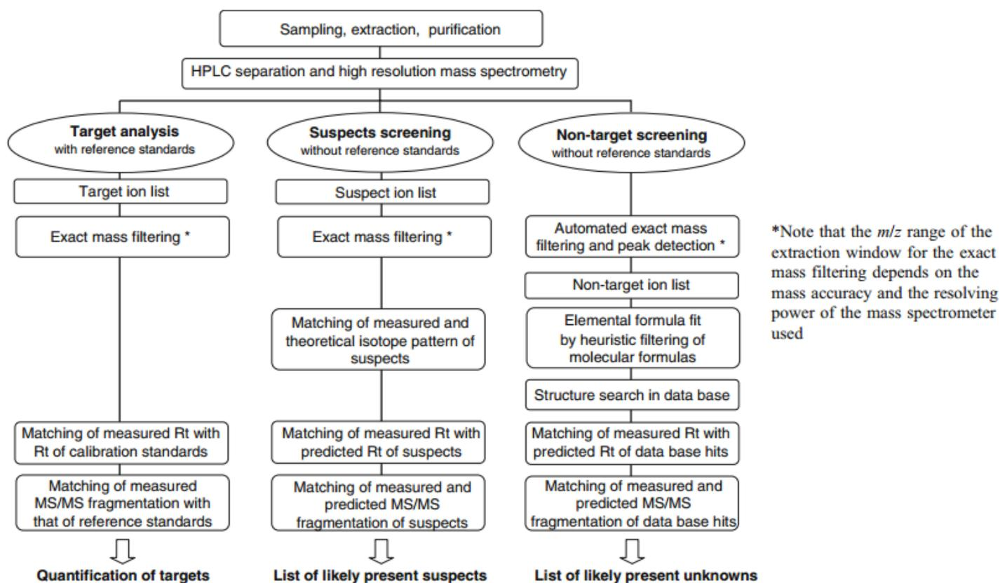
Figure 14: Systematic workflow for target, suspect and non-target screening by LC-HRMS/MS [48]
