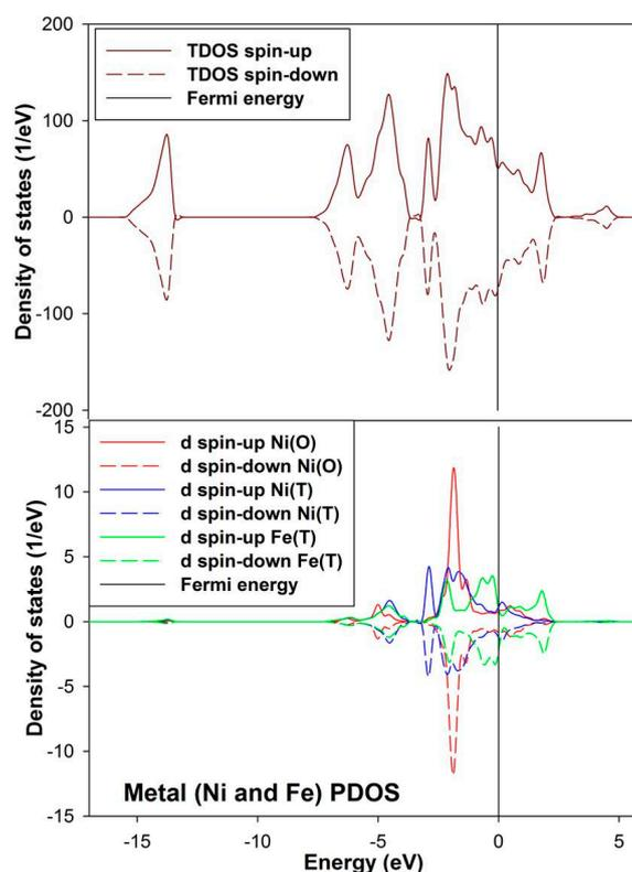
**Figure 4.** Projection total and partial density of states for the tetrahedral metals (Ni(T) and Fe(T)) and octahedral metals (Ni(O)) in the bulk conventional  $4(\text{Fe}_4\text{Ni}_5\text{S}_8)$  nickel-rich pentlandite.
