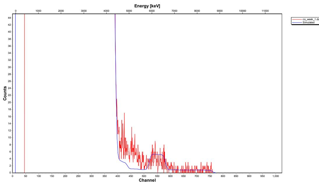
**Figure 6.**  $^{12}\text{C}$ -RBS spectrum of calcite  $\{10\bar{1}4\}$  interacted in an aqueous solution with a high  $\text{Co}^{2+}$  concentration ( $[\text{Co}_{\text{aq}}]_{\text{initial}} = 1000$  ppm) over one week.
