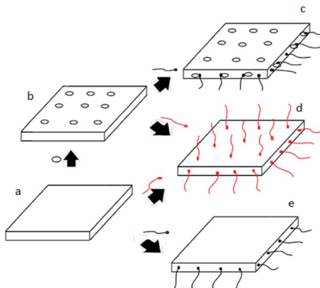
**Figure 11.** Schematic representation of the adsorption position of SDS and 1831 on the surface of MMT particles. (○:  $[\text{Cu}(\text{tetren})]^{2+}$ ; —: SDS; —: 1831).
