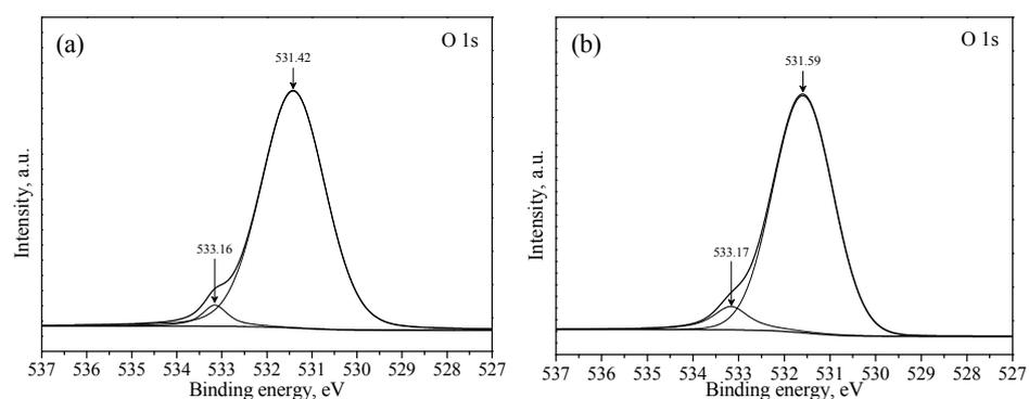
**Figure 4.** O 1s spectra for the mineral surface treated with chloride ions: (a) before; (b) after.
