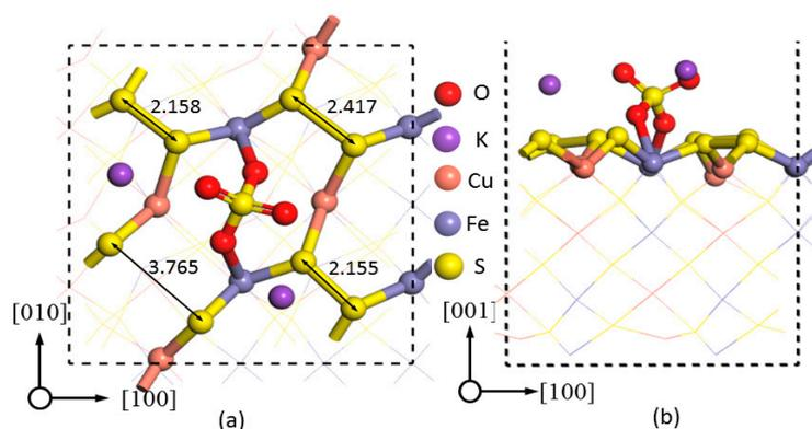
**Figure 8.** The most stable configuration of  $K_2SO_4$  adsorbed on the chalcopyrite (001)-S surface: (a) top and (b) side view in -BB mode. Distances are in angstroms.
