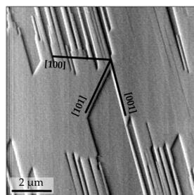
**Figure 1.** AFM image of a gypsum {010} surface dissolving in an undersaturated solution ( $\beta_{Gp} = 0.8$ ). Etch pits are oriented parallel to [001] and [101] and are  $\sim 7.5 \text{ \AA}$  in depth, which corresponds to the dimensions of half the  $b$ -axis periodicity of gypsum.
