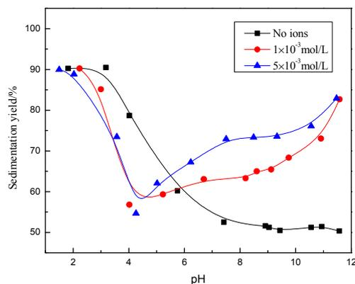
Figure 2. The effect of pH value on dispersion and flocculation of mineral with the presence of  $\text{Ca}^{2+}$ .
