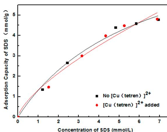
Figure 6. Adsorption capacity of SDS on the surface of original MMT sample and the MMT sample adsorbed with  $[\text{Cu}(\text{tetren})]^{2+}$ .
