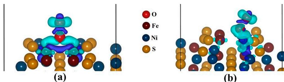
**Figure 10.** The sketch of isosurface charge density difference: (a) Fe-top site (isosurface level =  $0.004 \text{ e}\text{\AA}^{-3}$ ) and (b) Ni-top site (isosurface level =  $0.003 \text{ e}\text{\AA}^{-3}$ ). Cyan represents positive electronic clouds which accept electrons and blue stands for negative electronic clouds which donate electrons.
