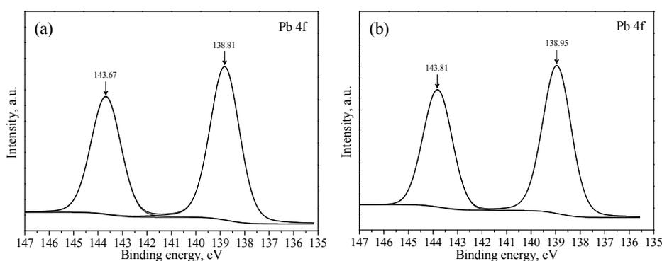
**Figure 5.** Pb 4f spectra for the mineral surface treated with chloride ions: (a) before; (b) after.
