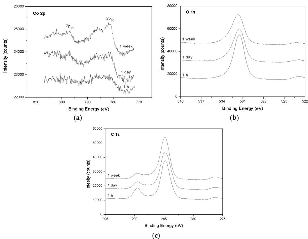
**Figure 4.** X-ray photoelectron spectra (XPS) spectra of calcite surfaces immersed in an aqueous solutions with a high Co<sup>2+</sup> concentration ( $[Co_{aq}]_{initial} = 1000$  ppm) for 1 h, one day and one week. (a) Co 2*p* (b) O 1*s* (c) C 1*s*.
