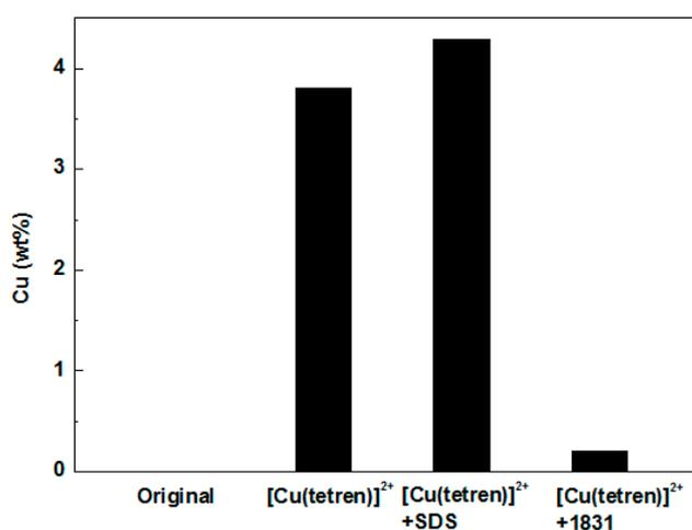
**Figure 8.** Content of Cu in MMT samples treated by different methods.
