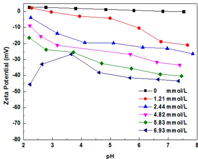
**Figure 9.** Zeta potential of MMT samples immersed in different concentration of SDS solutions with various pH values.
