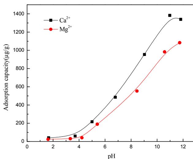
**Figure 9.** Adsorption capacity of Ca<sup>2+</sup> and Mg<sup>2+</sup> at different pH levels.
