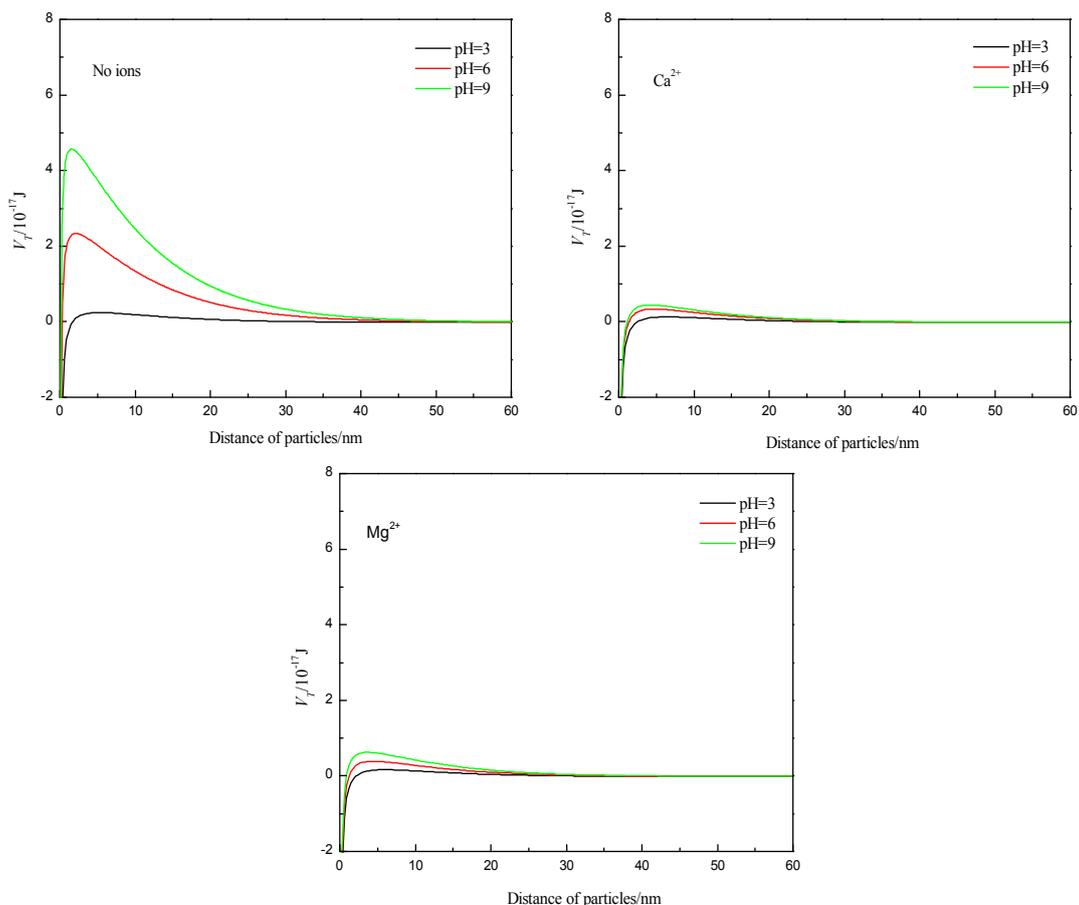
**Figure 5.** Total interaction energy of particles at different pH values without and with  $\text{Ca}^{2+}$ ,  $\text{Mg}^{2+}$ .
