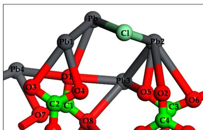
**Figure 6.** Adsorption configurations of  $\text{PbCl}^+$  on perfect cerussite (110) surface.
