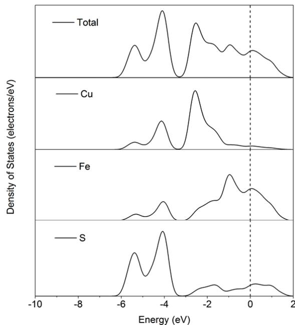
**Figure 4.** Density of states of chalcopyrite (001)-S surface.
