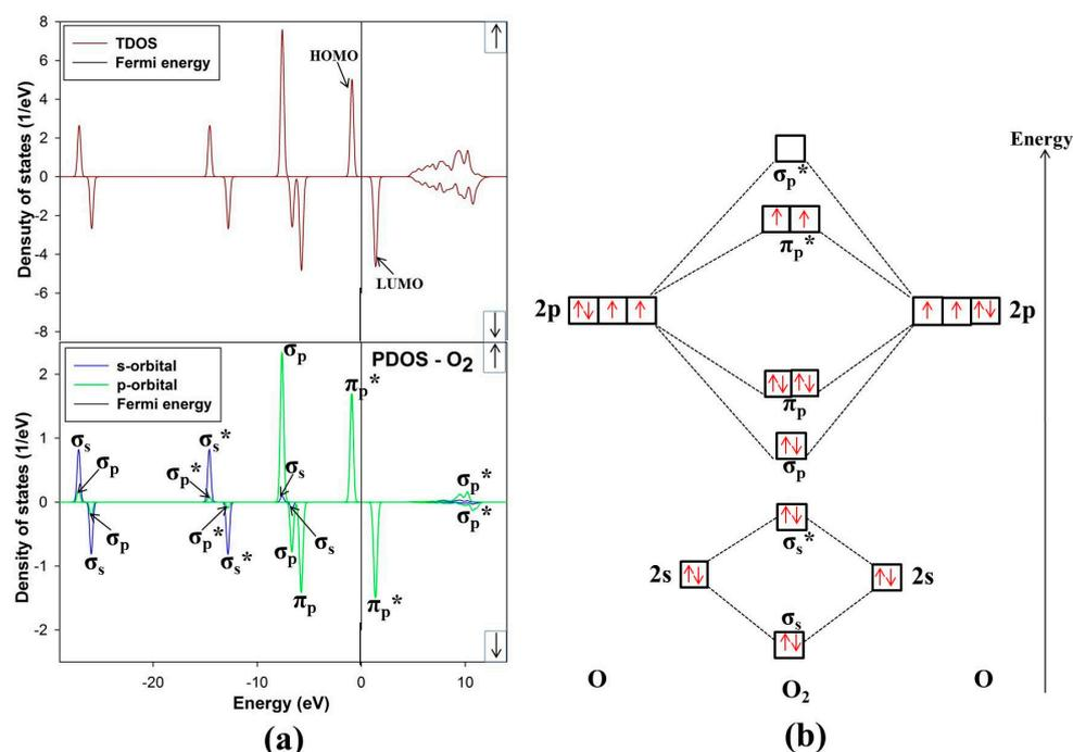
**Figure 6.** (a) Total and partial density of states and (b) molecular electron configuration of free O<sub>2</sub> molecule.
