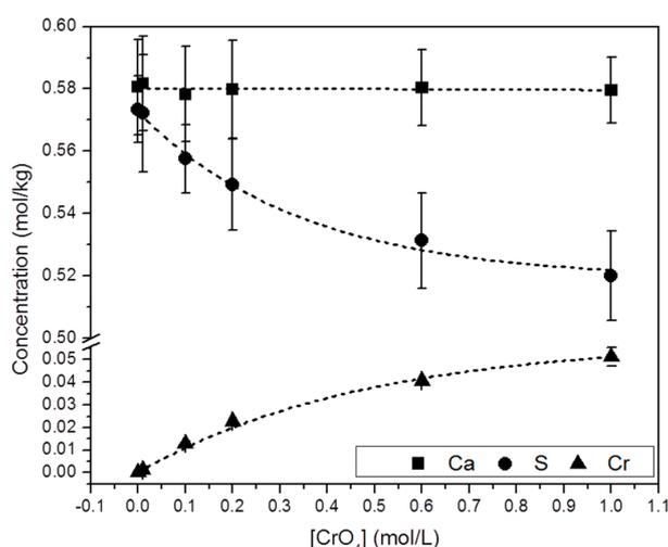
**Figure 5.** Chemical composition (from ICP-OES analyses) of solid samples collected from the precipitation experiments as a function of  $[\text{CrO}_4^{2-}]_{\text{aq}}$ . An increase of  $[\text{Cr}]_s$  is closely followed by a decrease in  $[\text{S}]_s$ . Analyses yielded similar  $[\text{Ca}]_s$  in all the solids.
