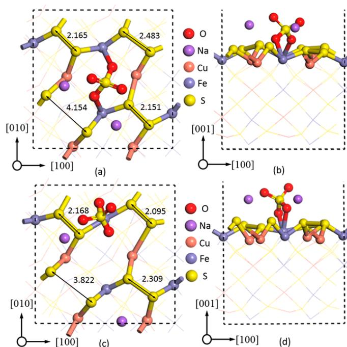
**Figure 7.** The most stable configuration of  $Na_2SO_4$  adsorbed on the (001)-S chalcopyrite surface: (a) top view and (b) side view in -BB mode; (c) top view and (d) side view in -BM mode. Distances are in angstroms.
