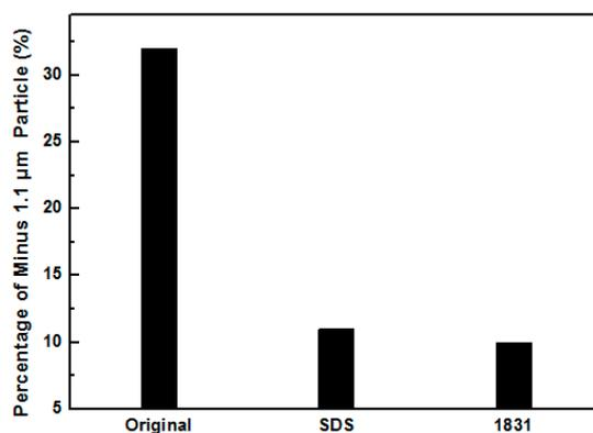
**Figure 3.** Stokes percentage of minus 1.1 μm particle in aqueous solutions pre-treated by of SDS and 1831.
