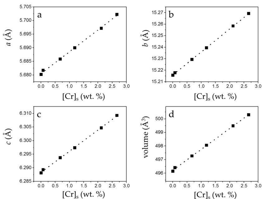
**Figure 7.** Unit cell parameters and cell volume (from the refinement of XRD patterns) of the precipitates plotted against  $[\text{Cr}]_s$ . Cell parameters (a–c) and cell volume (d) of gypsum increase as  $[\text{Cr}]_s$  increases.
