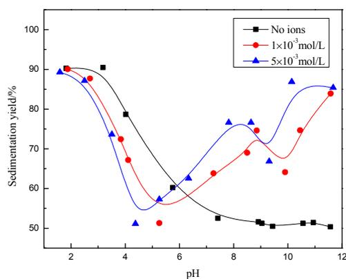
Figure 3. Effect of pH value on dispersion and flocculation of mineral with the presence of  $\text{Mg}^{2+}$ .
