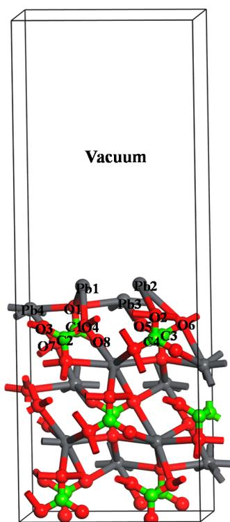
Figure 1. Slab model of perfect cerussite (110) surface.
