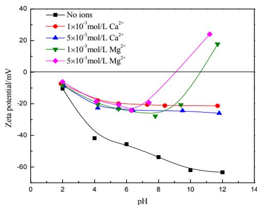
Figure 4. Zeta potentials of muscovite as a function of pH in deionized water with  $\text{Ca}^{2+}$  and  $\text{Mg}^{2+}$ .
