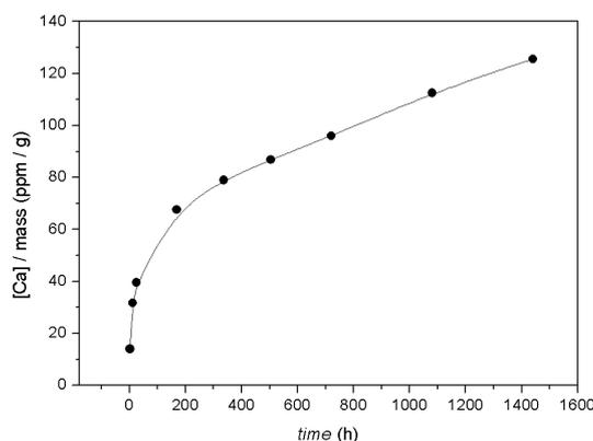
**Figure 3.** Release of  $\text{Ca}^{2+}$  (ppm of Ca per g of the solid) upon interaction of the powdered calcite with  $[\text{Co}^{2+}_{\text{aq}}]_{\text{initial}} = 1000$  ppm as a function of time.
