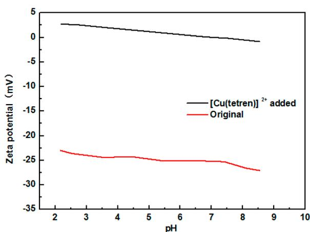
Figure 5. Zeta potential of MMT treated with  $[\text{Cu}(\text{tetren})]^{2+}$ .
