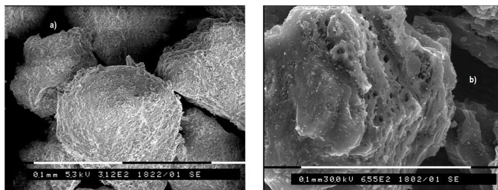
**Figure 1.** Examples of powder particles with high SSA: fractal-like topography of montmorillonite (a) with  $SSA \approx 1000 \text{ m}^2 \cdot \text{g}^{-1}$  (nanometric pores) and activate black coal (b) with surface area around  $1100 \text{ m}^2 \cdot \text{g}^{-1}$  and pore size of approximately  $5 \mu\text{m}$  (maximum)—its surface seems to be non-homogenous, *i.e.*, non-fractal. Scale bars 0.1 mm.
