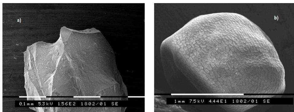
**Figure 2.** Relatively smooth surface topography of olivine,  $SSA \approx 1 \text{ m}^2 \cdot \text{g}^{-1}$  (a) and bio-sample of rapeseed oil having bio-topography (b)—where the surface area was not measured. Scale bars: (a) 0.1 mm, (b) 1 mm.
