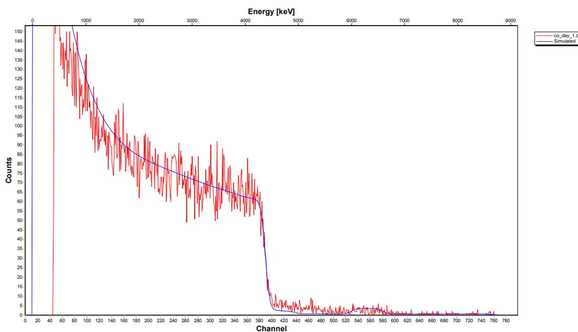
**Figure 5.**  $^{12}\text{C}$ -RBS spectrum of calcite  $\{10\bar{1}4\}$  interacted in an aqueous solution with a high  $\text{Co}^{2+}$  concentration ( $[\text{Co}_{\text{aq}}]_{\text{initial}} = 1000 \text{ ppm}$ ) over one day.
