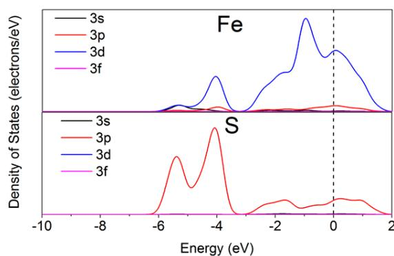
**Figure 5.** Partial density of states of chalcopyrite (001)-S surface.
