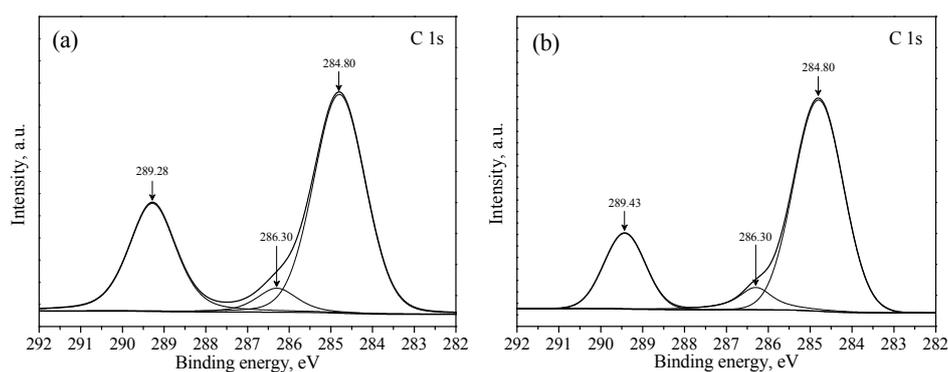
**Figure 3.** C 1s spectra for the mineral surface treated with chloride ions: (a) before; (b) after.
