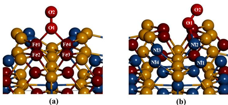
**Figure 8.** The relaxed geometries of O<sub>2</sub> molecule on the surface: (a) fcc-hollow site and Fe-top site and (b) Ni-top site.
