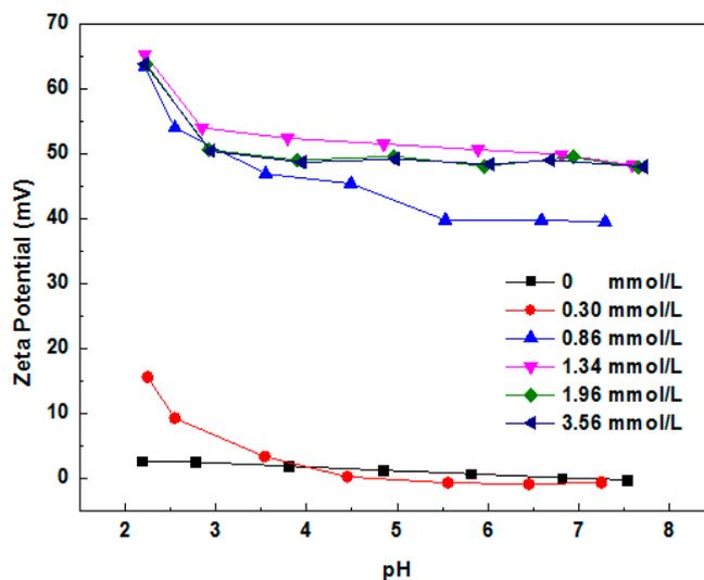
**Figure 10.** Zeta potential of MMT samples immersed in different concentrations of 1831 solutions with various pH values.
