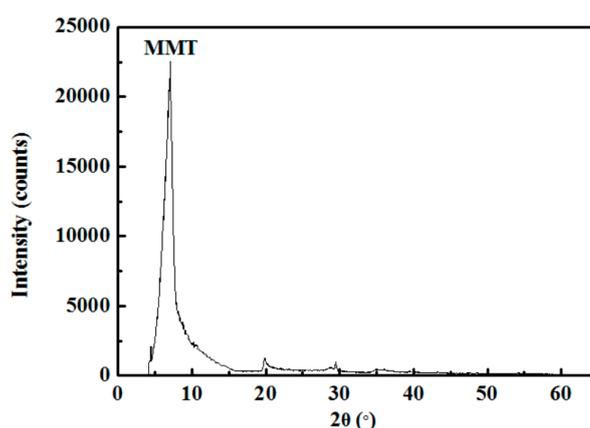
Figure 1. XRD pattern of MMT sample.
