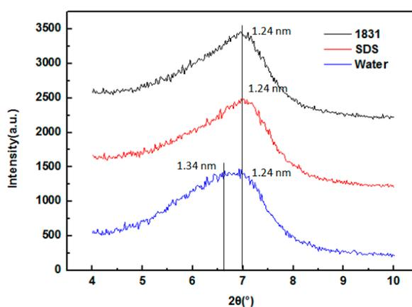
**Figure 4.** XRD pattern of MMT particles pre-treated by mechanical chemical adsorption of SDS and 1831.
