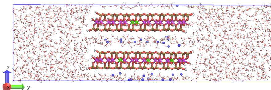
**Figure 2.** Simulation cell and initial atomic configuration of Na-MMT AC edge at  $t = 0$ . The Al atoms are magenta; Mg atoms are green; Si atoms are ochre, O atoms are red, H atoms are white, and Na atoms are blue.
