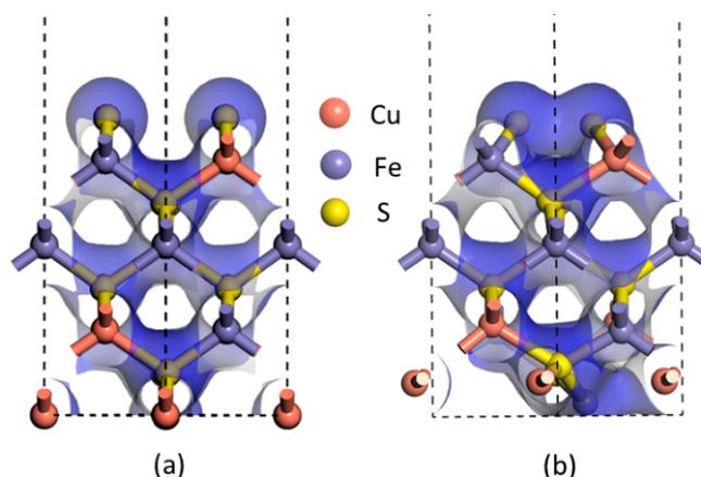
**Figure 3.** The electron density of chalcopyrite (001)-S surfaces: (a) unrelaxed and (b) relaxed.
