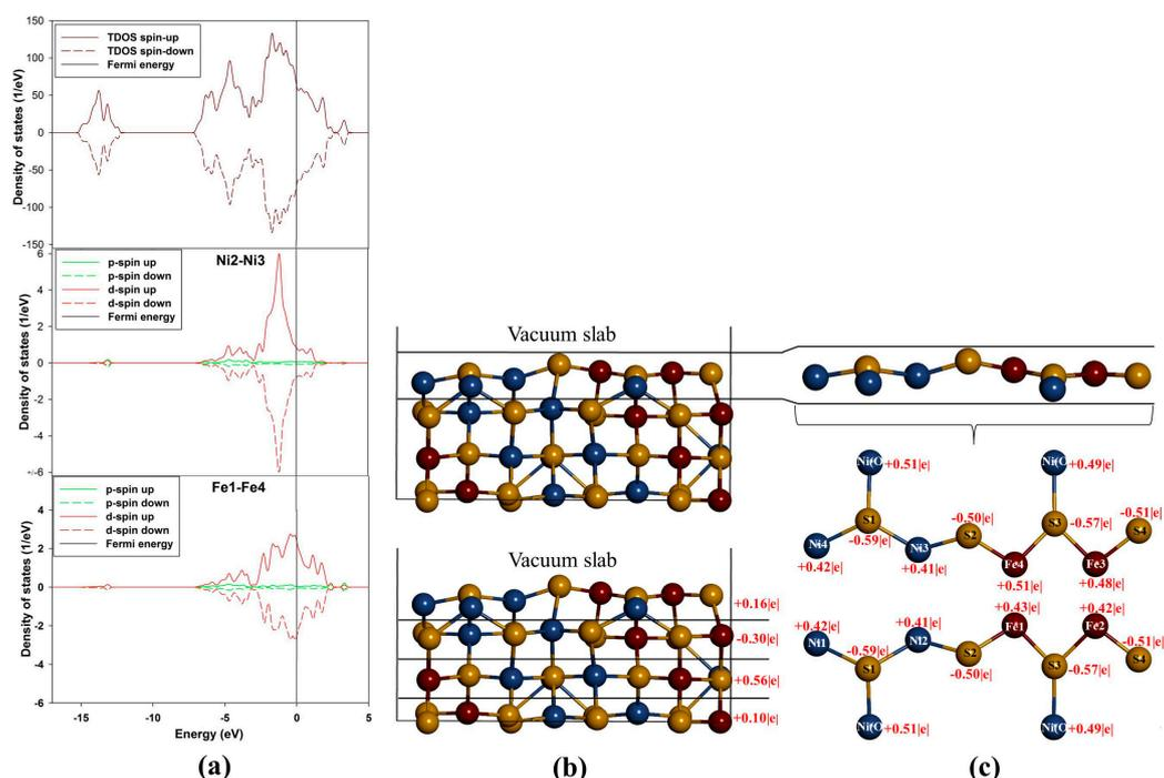
**Figure 5.** Projection density of states and Bader charges for the top adsorbed Ni and Fe atoms: (a) total and partial density of states; (b) Bader charges for each layer and (c) Bader charges for the top layer atoms.
