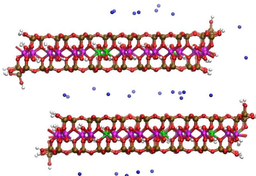
**Figure 6.** Snapshot of the Na-MMT MD simulations shown in profile at  $t \sim 3.5$  ns; water molecules removed for clarity. Disordered structures have developed at the AC edge interfaces. The Al atoms are magenta; Mg atoms are green; Si atoms are ochre, O atoms are red, H atoms are white, and Na atoms are blue.
