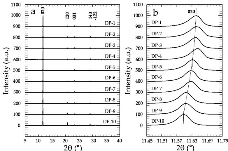
**Figure 6.** (a) Powder X-ray diffraction patterns of the precipitates. For the sake of clarity, all of the diffractograms have been normalized to the (010) peak, which is the most intense reflection; (b) Magnification of the (020) reflection, where a clear shift of this reflection towards lower  $2\theta$  values as  $[\text{Cr}]_{\text{aq}}$  increases can be observed.
