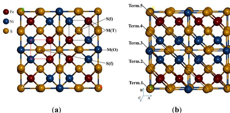
**Figure 1.** The crystal structure of nickel-rich pentlandite: (a) conventional  $4(\text{Fe}_4\text{Ni}_5\text{S}_8)$  and (b) different terminations considered. M(O) and M(T) represent the octahedral and tetrahedral metals, respectively, with S(f) and S(l) representing the face-capping and the linked sulphurs, respectively.
