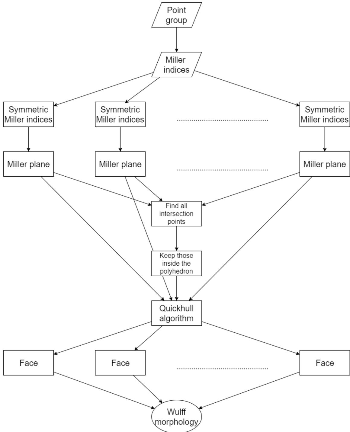
Figure 33: The workflow for the construction of the Wulff morphology.
