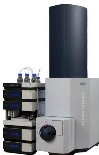
**Figure 10: UHPLC-QToF-MS, Maxis Impact, Bruker Daltonics**
