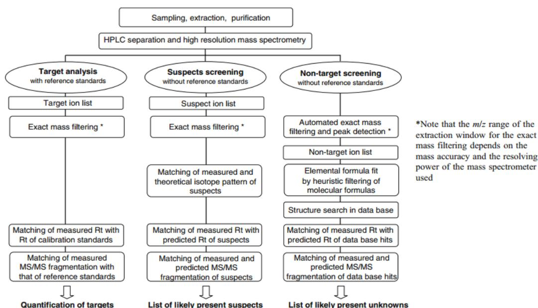
**Figure 7: Systematic workflow for target, suspect and non-target screening by LC-HRMS/MS [60]**
