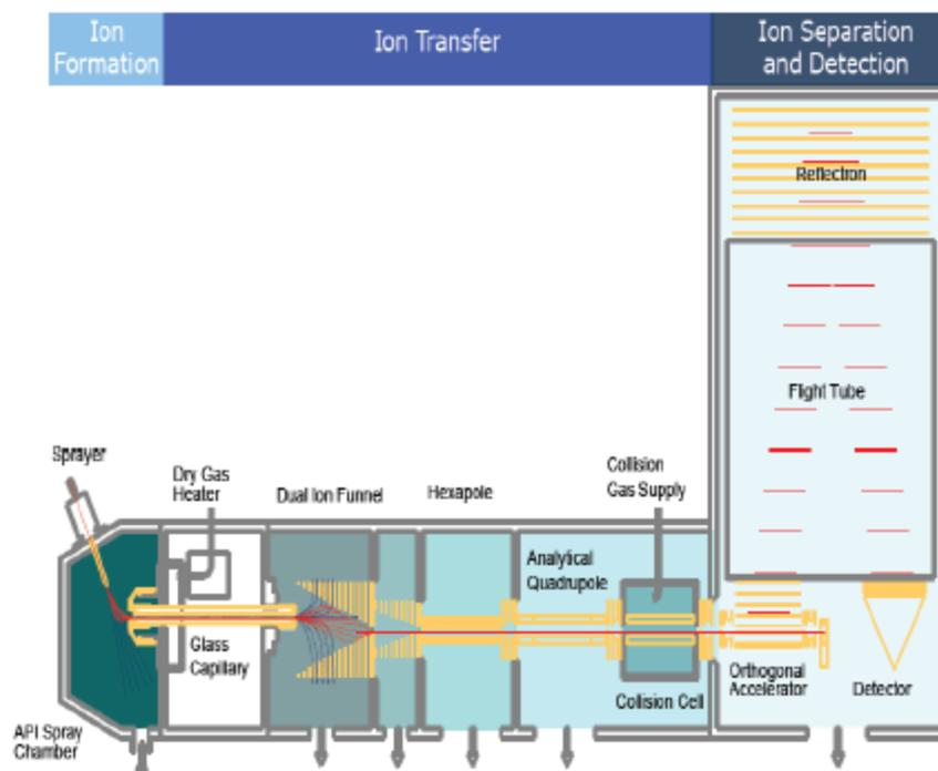
**Figure 6: Course of ions in the QTOF sections (maXis Impact, Bruker)**
