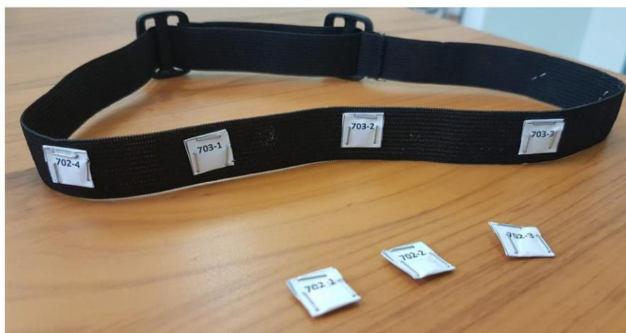
**Fig. 3.3.2** A set of 7 TLDs that were used on this study
