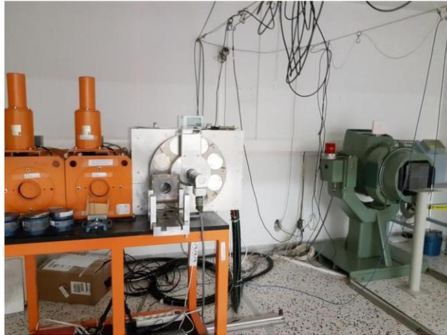
**Fig. 3.3.9 PANTAK X-ray tube at the Ionizing Radiation Calibration Laboratory of the Greek Atomic Energy Commission**
