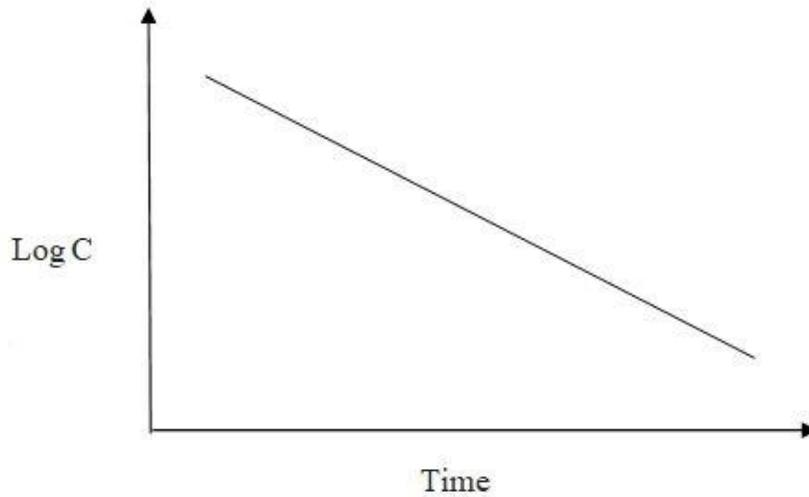
**FIGURE 3. TIME PROFILE OF A ONE-COMPARTMENT MODEL SHOWING THE LOG CONCENTRATION (C) VERSUS TIME.**
