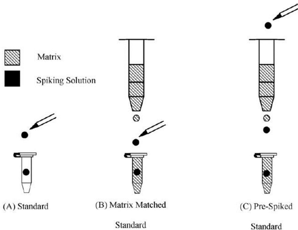
**Figure 23. Preparation of solutions for the determination of recovery rate and matrix effect, source:[99]**
