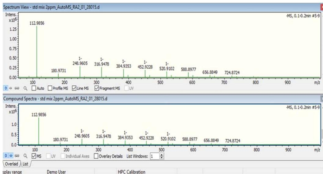
**Figure 14. The mass spectrum of calibrant after calibration**
