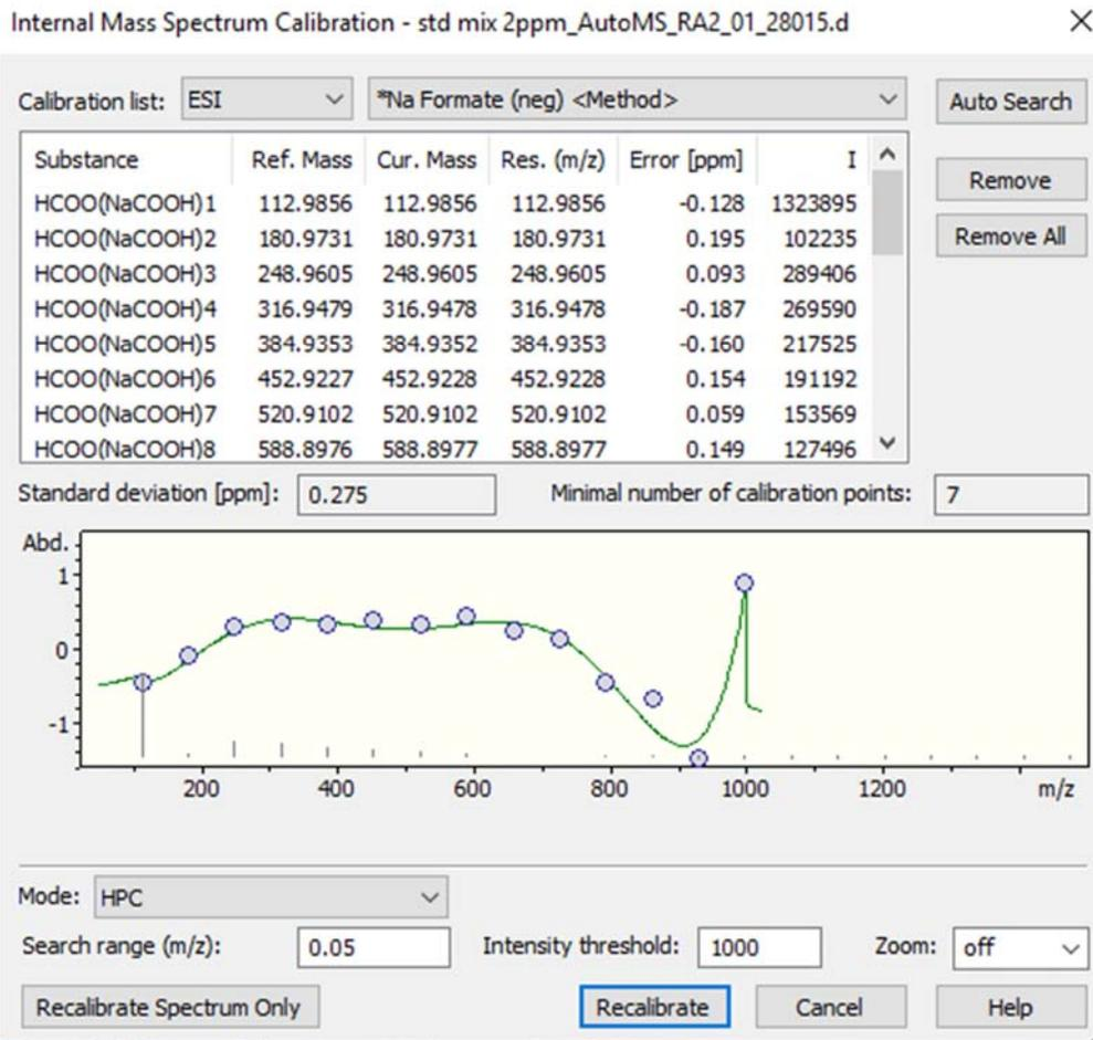
Figure 13. Internal calibration of mass spectrum.
