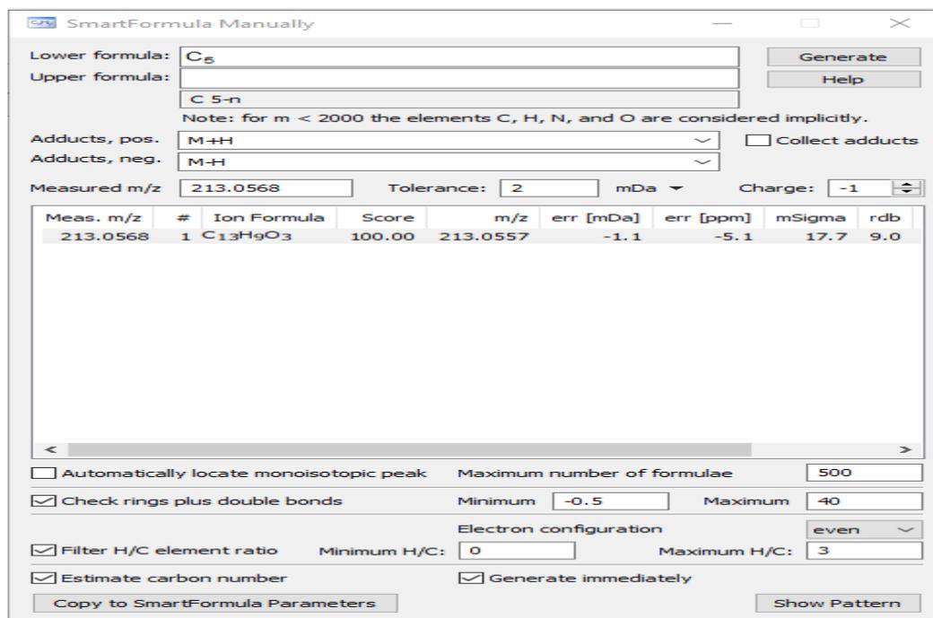
Figure 20. Assignment of possible elemental composition using “SmartFormula Manually” for one of the fragments
