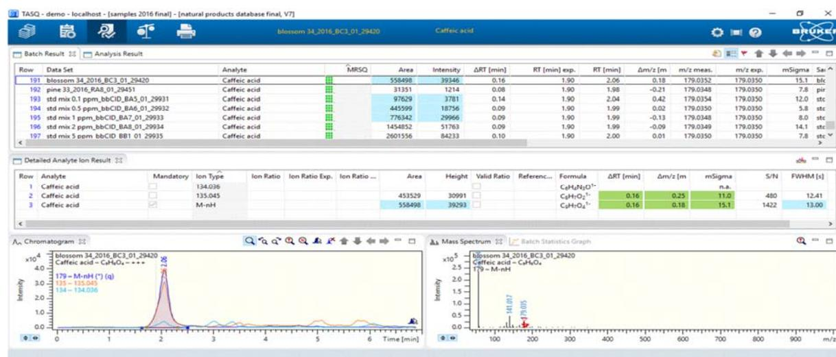
Figure 24. Target screening of samples for the determination of caffeic acid
