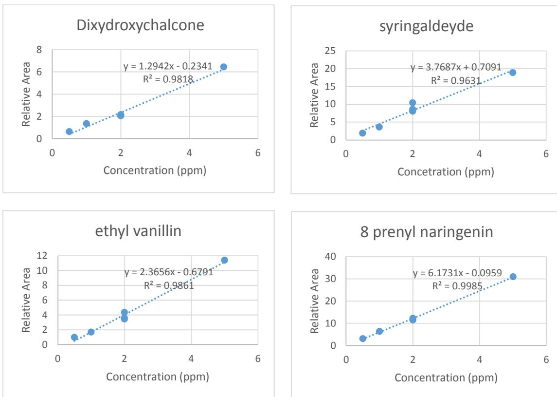
Figure 21. The selection of internal standards for chrysin based on the calibration curves.
