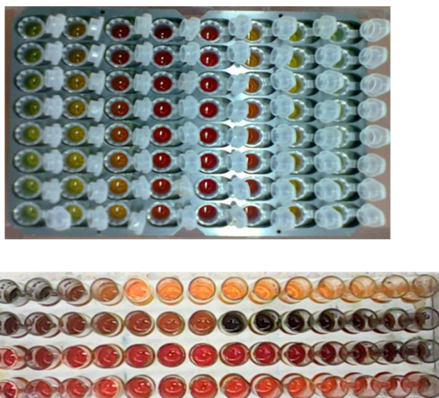
Figure 16: CPC fractions from semi-prep CPC (up) and prep-CPC (down) indicating the power of CPC technique to efficiently separate, enrich and purify complex mixtures of natural compounds
