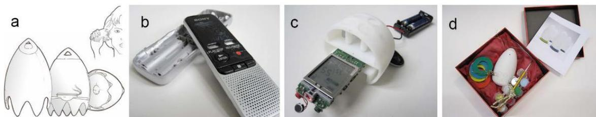
**Figure 5: Example of cracking it open prototype: A Dictaphone provided the functionalities of a sound bauble. Image from project: Digital Christmas Memories [15].**
