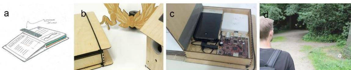
**Figure 6: Example of a collating prototype: An embedded computer and a Bluetooth speaker create interactive location-based audio in the cemetery. Image from project: Interactive Cemetery [15].**
