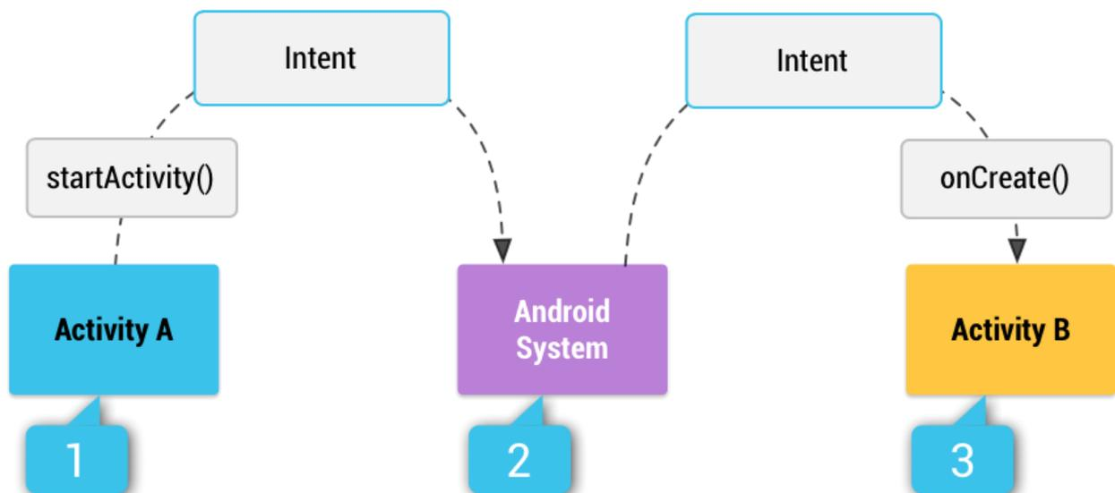
**Figure 47: How an implicit intent is delivered through the system to start another activity: (1) Activity A creates an Intent with an action description and passes it to `startActivity()`. (2) The Android System searches all apps for an intent filter that matches the intent. When a match is found, (3) the system starts the matching activity (Activity B) by invoking its `onCreate()` method and passing it the Intent.**
