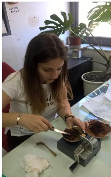
**Figure 3.8.2:** Applying the method to measure the liquid limit.
