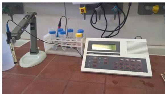
**Figure 3.6:** The pH meter (JENWAY 3040 Ion Analyser) at the laboratory of Economic Geology and Geochemistry, NKUA.
