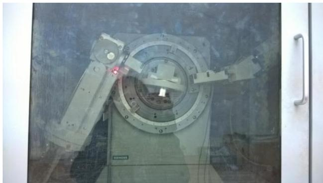
**Figure 3.2:** X-ray diffraction instrument (SIEMENS D5005 X-RAY DIFFRACTIONMETER) at the laboratory of Economic Geology and Geochemistry, NKUA.
