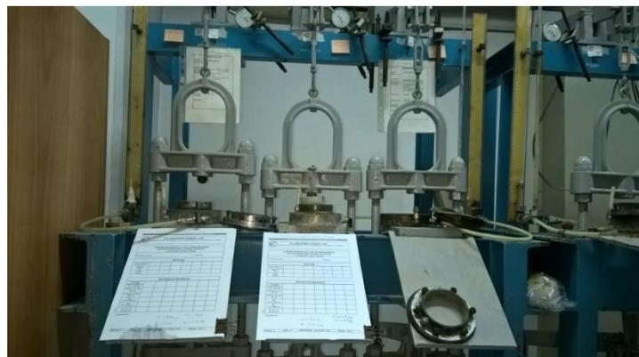
**Figure 3.8.1:** The oedometer device, at the laboratory of Edafomichaniki S.A.
