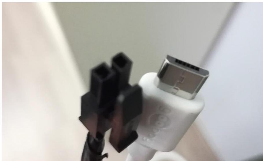
Figure 12: Cable that powers the Raspberry from TurtleBot's battery
