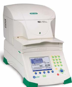
Figure 6. A typical thermal cycler machine for RT-PCR
