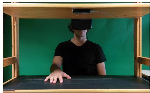
**Figure 2.21:** Experimental setup. User wearing HMD, Leap motion on top.
