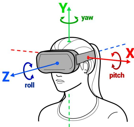
**Figure 2.10: The six degrees of freedom. Three positional axis and three rotational [43].**
