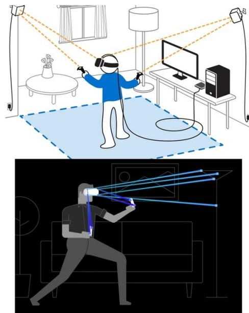
**Figure 2.11: Tracking (Top) Outside-in [15]. (Bottom) Inside-out [11].**
