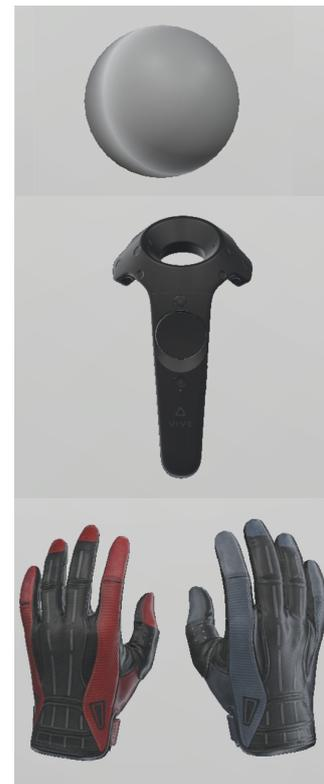
**Figure 3.3: Three different virtual hand representations. (Top) Sphere (Middle) Controller (Bottom) Hand.**
