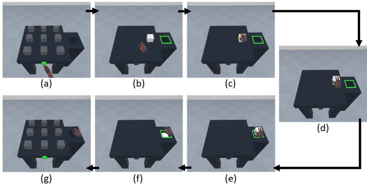
**Figure 3.1:** The steps of the task are (a) users push the green virtual button, (b) one cube becomes non-transparent, (c) they approach and touch it, (d) they grab it by pressing the trigger, (e) they position it to the hole, (f) they place it inside the hole, (g) table gets reset for the next task.
