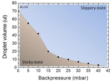
**Figure 2.** Effect of the backpressure on the mobility of water droplets of various volumes at porous surfaces with holes tilted at 0 $^{\circ}$ .
