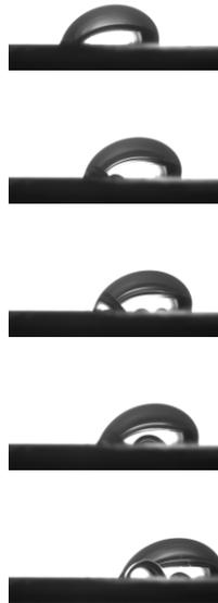
**Figure 3.** A 60  $\mu\text{l}$  water droplet tilted at 30 deg, is moving upon backpressure application.
