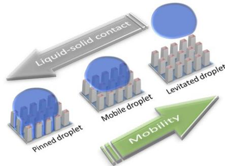
**Figure 1.** Schematic representation of a droplet exhibiting various wetting states, corresponding to different mobility states of the surface.
