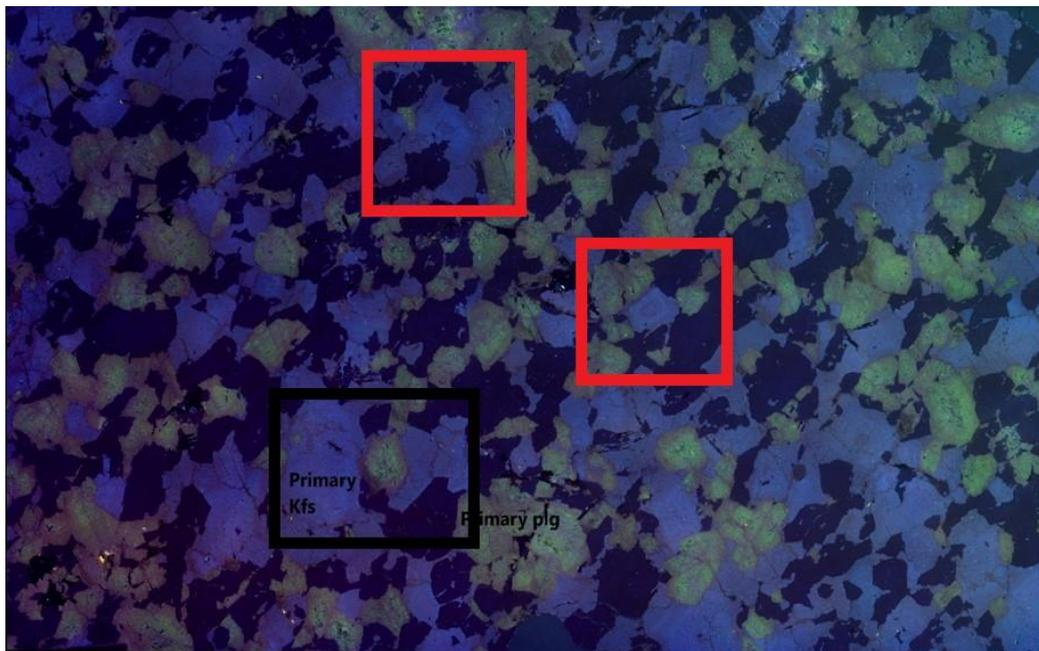
Fig.30: CL image of the unaltered aplogranite from Sotiras area. Both the plagioclase and the K-feldspar are fresh showing oscillatory zoning (see following figure).
