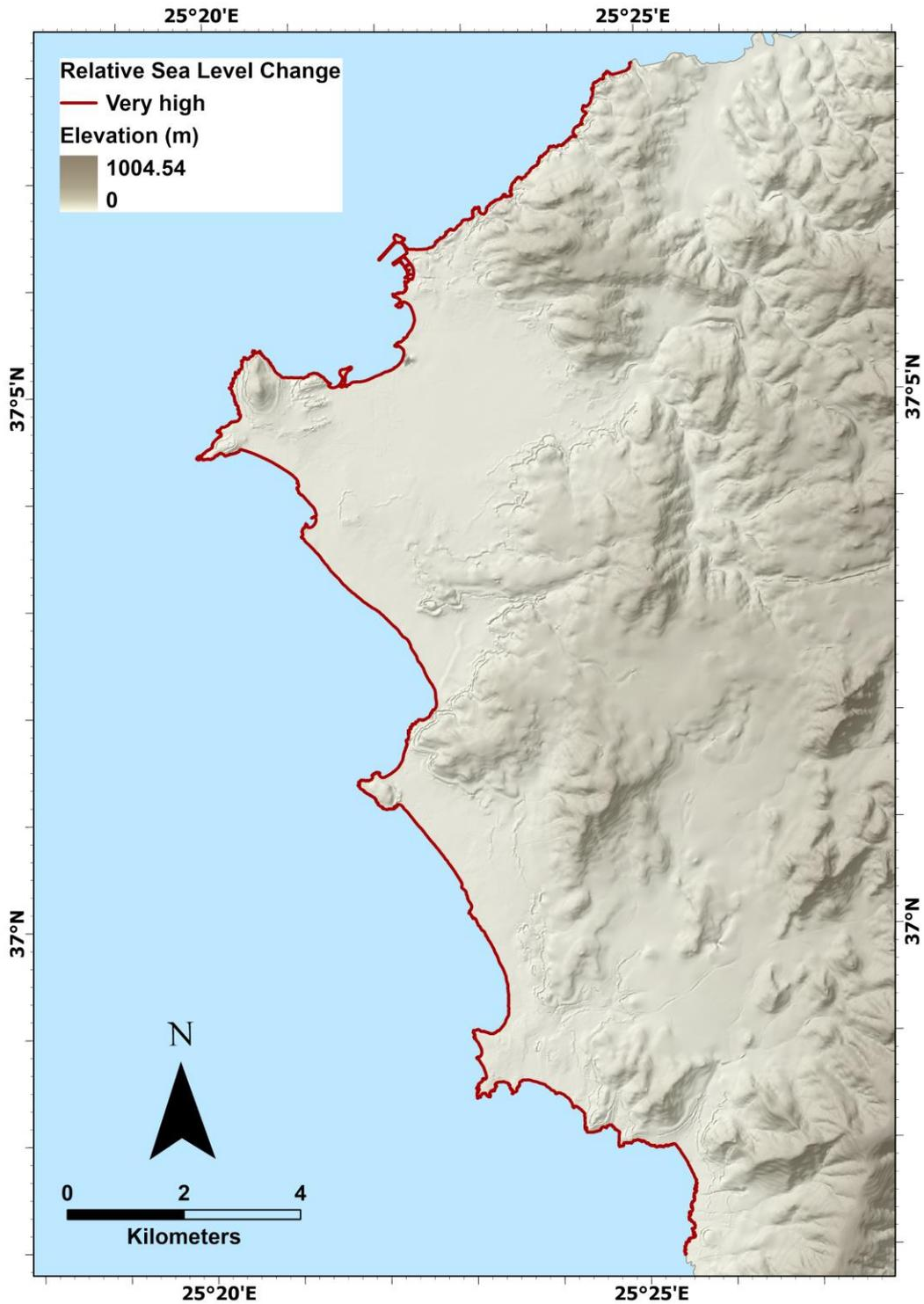
Figure 17: Map of vulnerability classification of the western Naxos coastline, according to the variable of Relative Sea Level Change.
