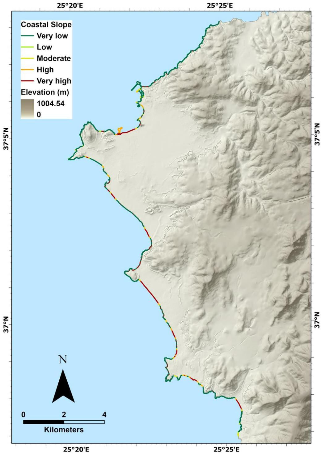
Figure 16: Map of vulnerability classification of the western Naxos coastline, according to the variable of coastal slope.
