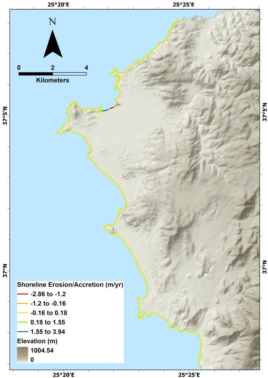
Figure 18: Map of vulnerability classification of the western Naxos coastline, according to the variable of Shoreline Erosion/Accretion rates.
