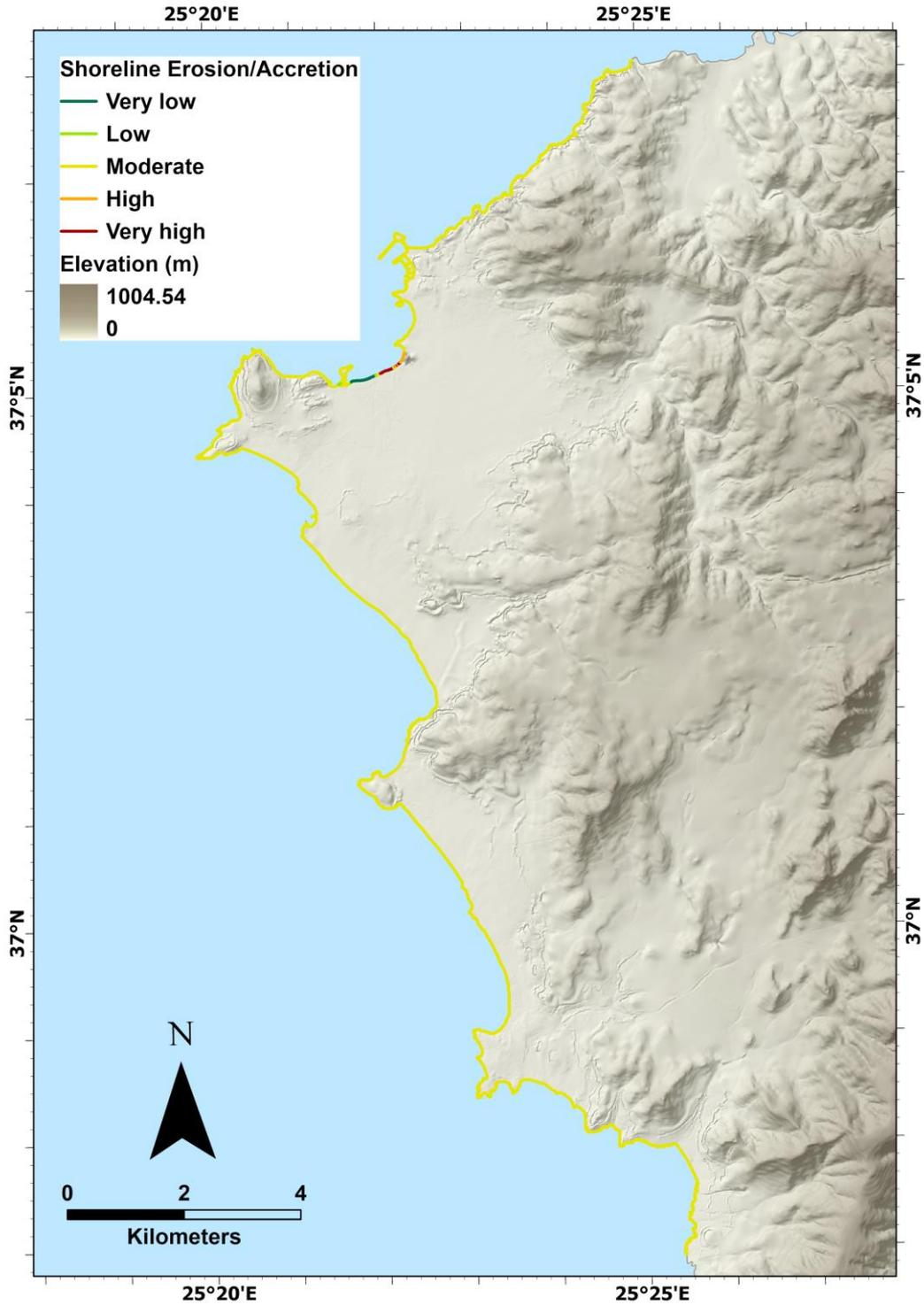
Figure 19: Map of vulnerability classification of the western Naxos coastline, according to the variable of Shoreline Erosion/Accretion.
