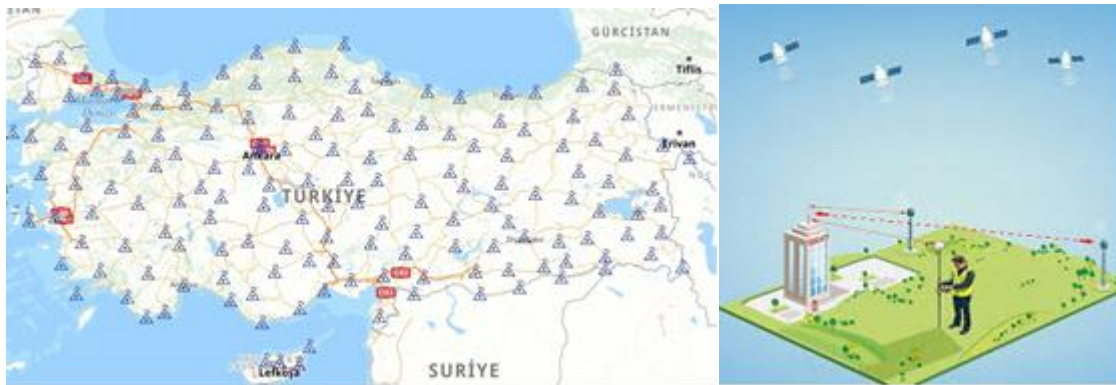
Image 25 The TUSAGA - AKTIF with its 146 reference stations that are synchronized with the remote and the satellites.
