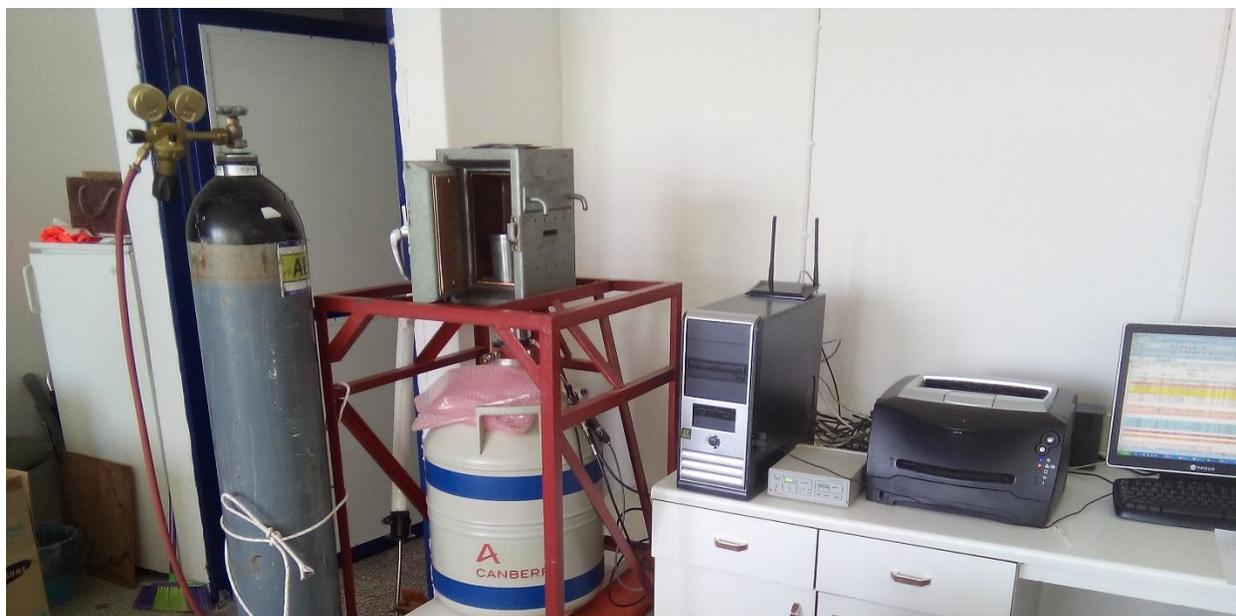
**Fig. 10:** The  $\gamma$ -ray spectrometry system
