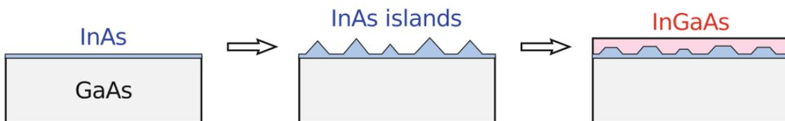
**Figure 3-9 : The Stranski – Krastanov method. Growth of a InAs thin layer upon a GaAs substrate by means of epitaxy. The height of the InAs at this point is equal only to a few atoms (left). Further growth leads to the spontaneous emergence of isolated pyramidal islands known as QDs (middle). Overgrowth of these islands with a InGaAs layer flattens then QDs and results in a DWELL structure [55].**
