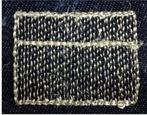
Figure 1-4. Embroidered meshed microstrip patch antenna on denim base fabric [6].
