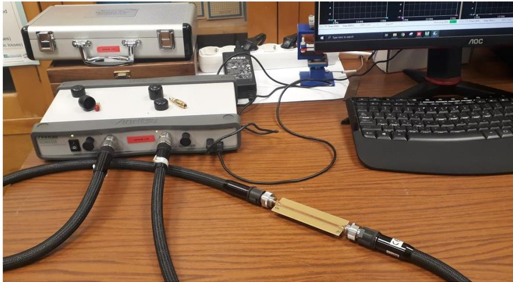
Figure 4-3. Microstrip line measurement set-up.
