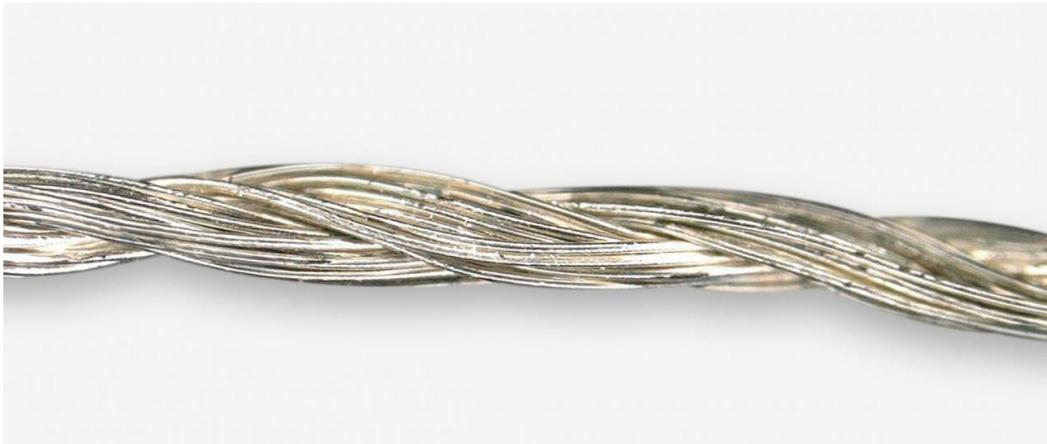
Figure 3-10. Close up of the Shieldex 117/17 2-ply conductive thread [3].
