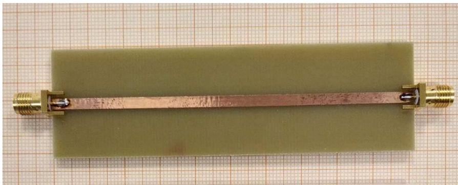
Figure 4-2. Prototype of reference copper microstrip line.
