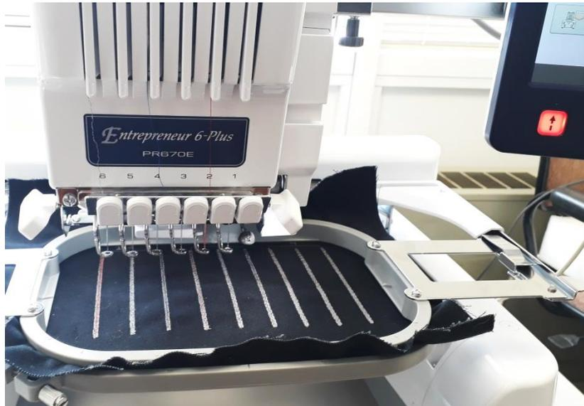
Figure 4-10. Embroidered lines on frame after the completion of the embroidery process.
