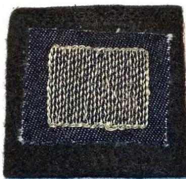
Figure 3-20. Embroidered non-uniform, meshed microstrip patch antenna [4].
