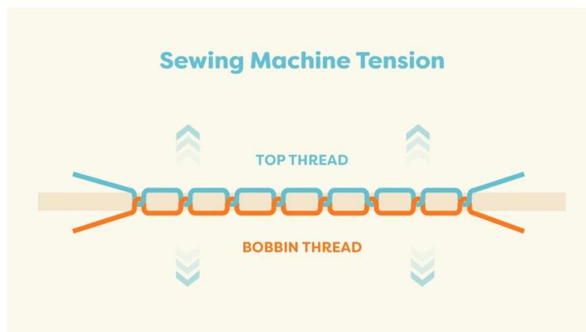
Figure 3-13. Visualization of top and bobbin thread tensions [23].
