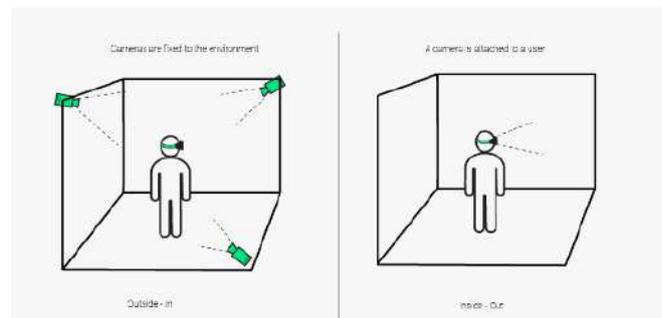
Figure 2.11: Outside-in and Inside-out tracking [20].
