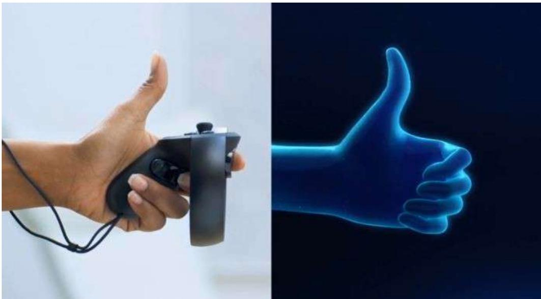
**Figure 2.12: On the left side is the controller of Oculus Quest and on the right side the projection of the virtual hand**
