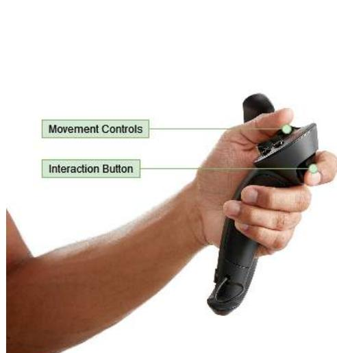
Figure 3.15: Controls in the Valve Knuckles Controller
