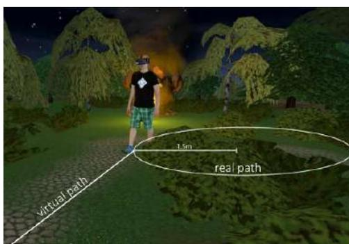
**Figure 2.17: TeleWalking an RDW technique [53].**
