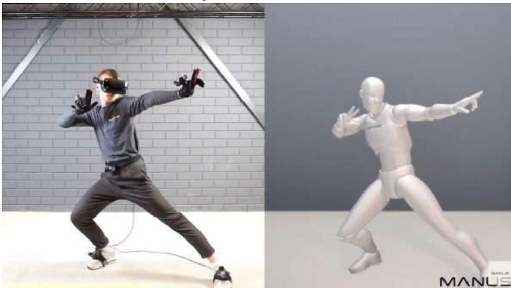
Figure 2.14: Full body tracking using Vive Trackers [Manus] [49].
