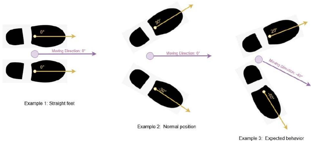
**Figure 3.2: Feet-based direction method: 3 example of how the moving direction is calculated**
