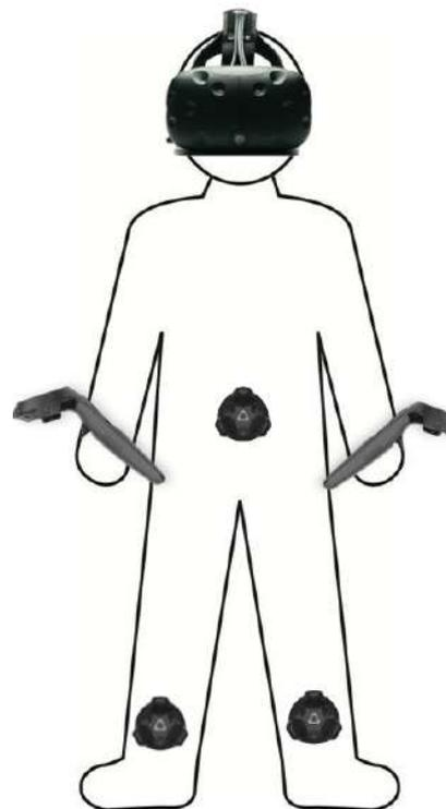
**Figure 3.1: Equipment over the body of the user. The extra hardware consists of three Vive Trackers, one placed in the area of the Hip and two others over the feet.**
