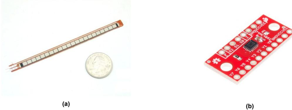
Figure 9: (a) A thick laminate flex sensor. (b) An IC analog multiplexer device.
