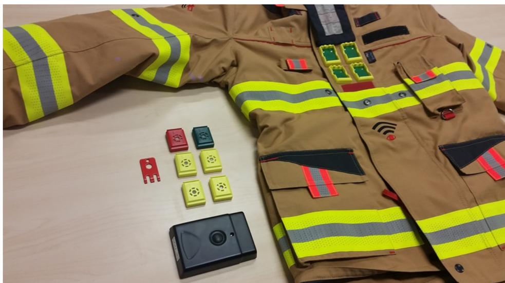
**Figure 3.12: Sensors in the suit of the firefighters [44]**
