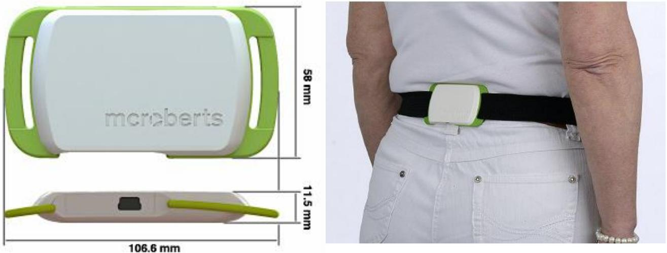
**Figure 2:** DynaPort MoveMonitor; McRoberts B.V., The Hague, The Netherlands (106.6x58x11.5mm, 55 grams; range  $\pm 6$  g, sampling frequency: 100Hz) and its positioning at the level of the L2 vertebra.
