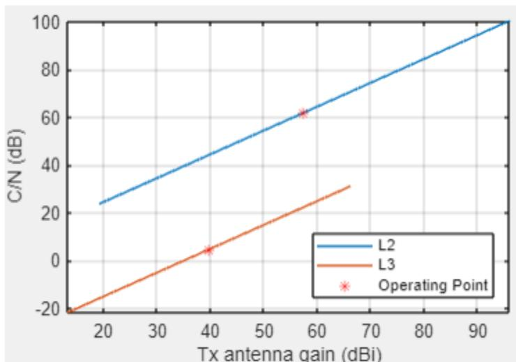
**Figure 25:  $C/N$  relative to transmitting antenna gain****6.4.2.3.5  $C/N_o$  and frequency metrics**
