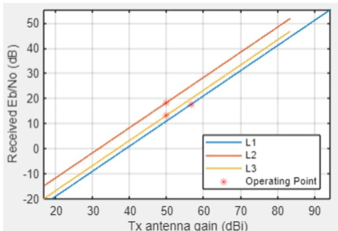
Figure 15: SNR-per-bit and antenna gain comparison
