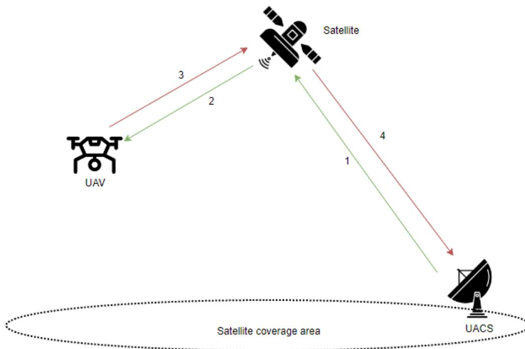
**Image 54: Links for BLoS with satellite as relay**
