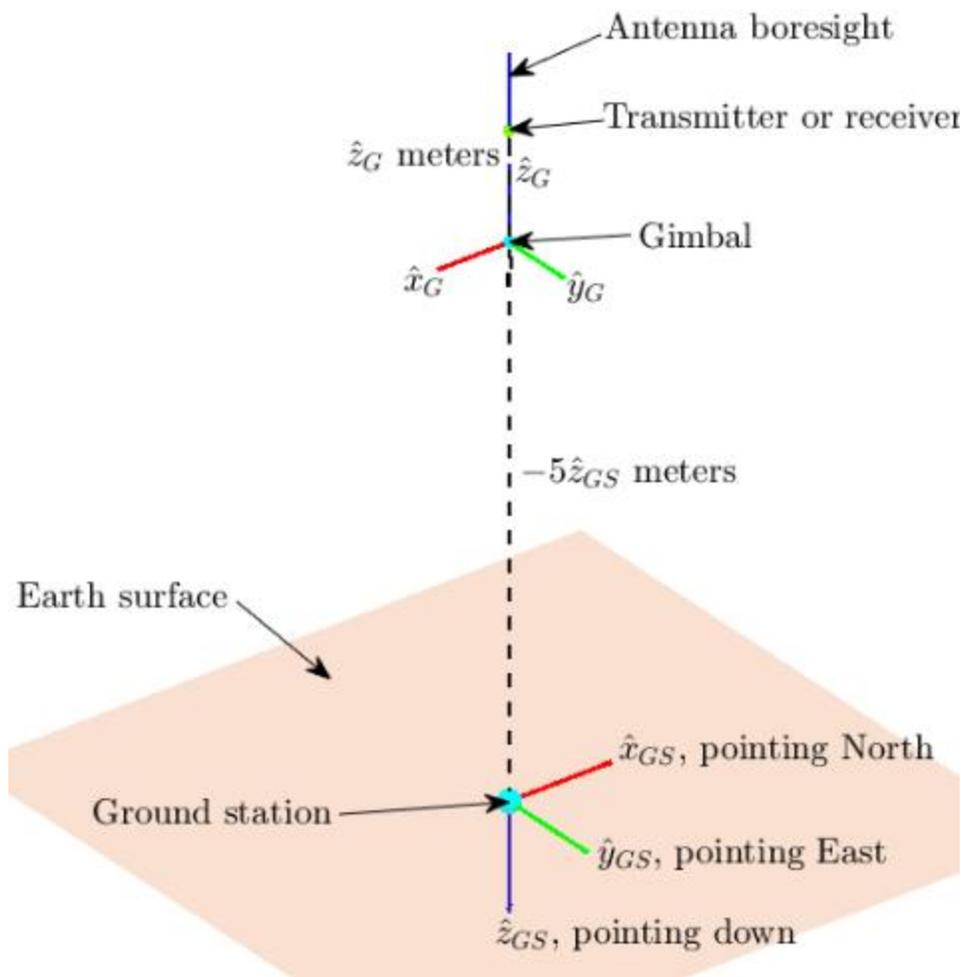
**Image 37: Cartesian coordinates for both gimbal and transmitter/receiver for the ground station**
