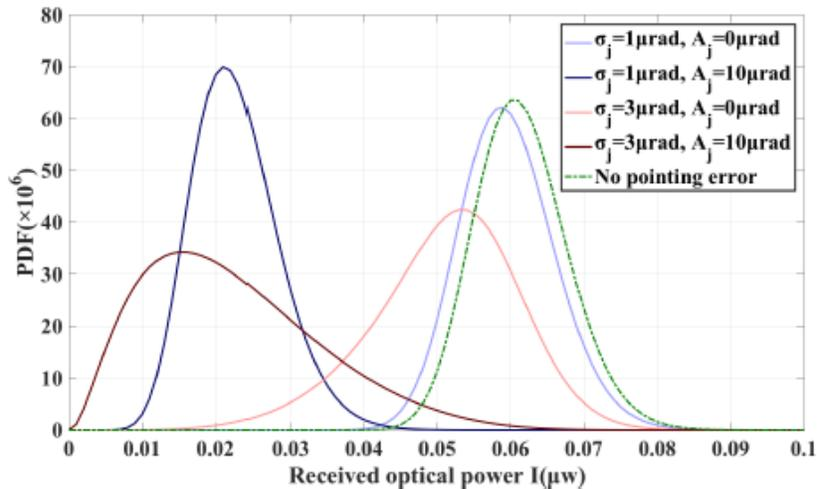
**Figure 5: PDF for both pointing and no-pointing error for uplink channel**
