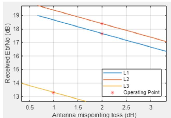
Figure 16: SNR-per-bit and antenna mispointing loss comparison
