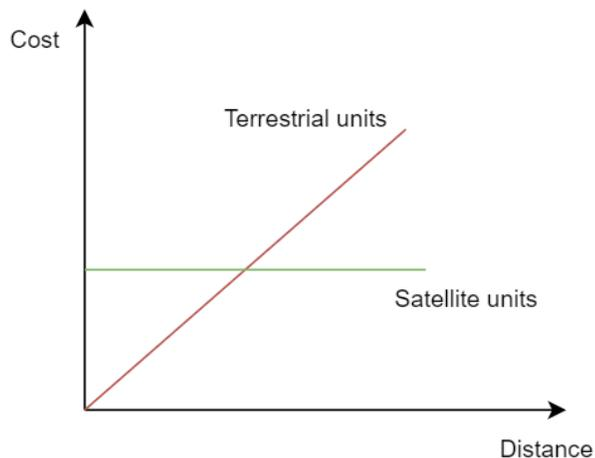
**Figure 4: Terrestrial vs satellite cost and distance**
