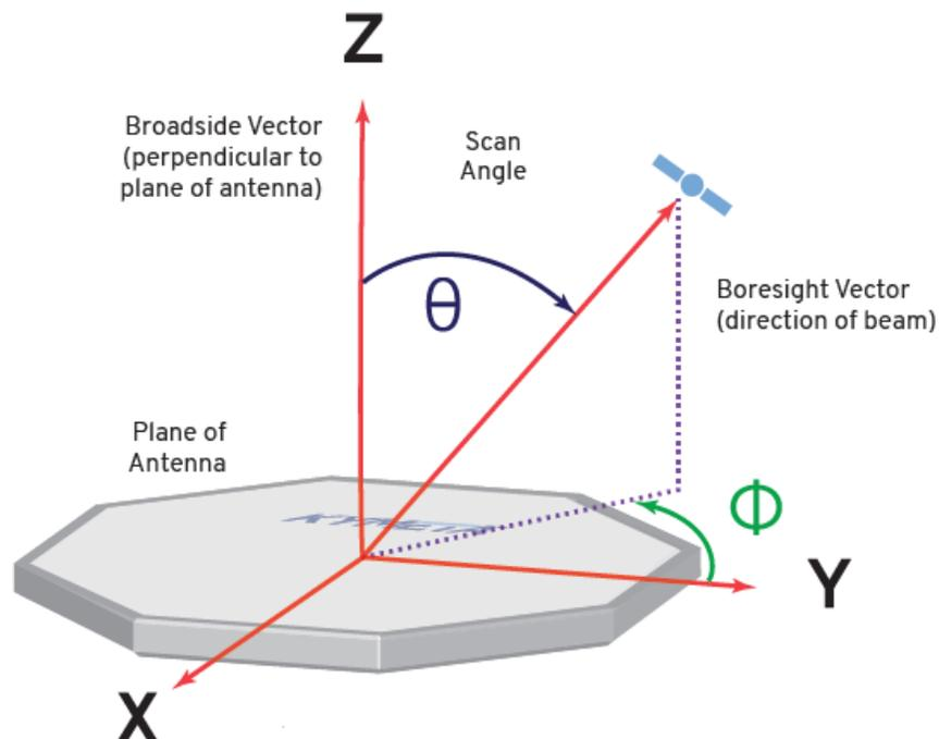
Image 41: Configuration for the gain of the antenna [72]
