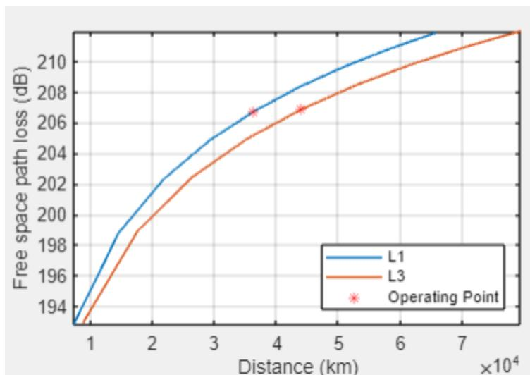
Figure 19: Free space path losses relative to distance
