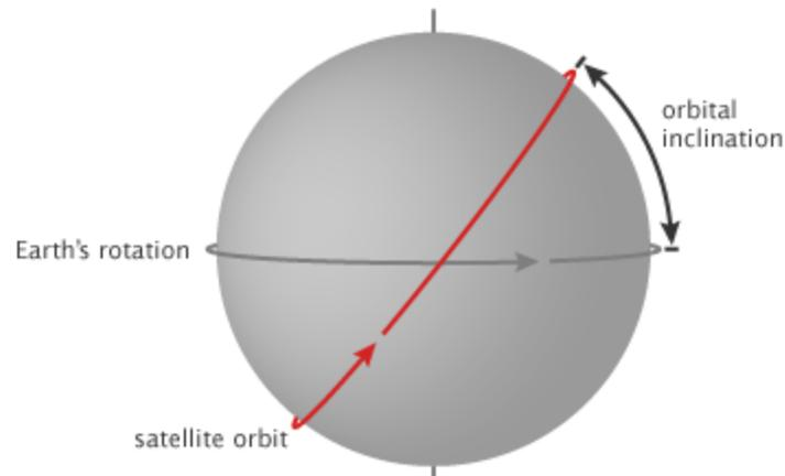
**Image 31: Inclination of an orbit [68]**
