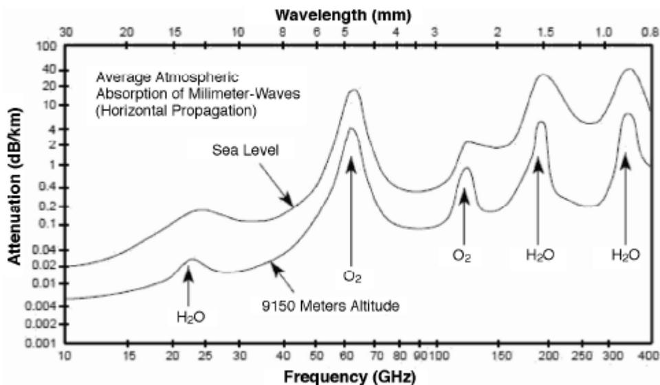
Figure 8: Atmospheric loss relative to frequency and wavelength [72]
