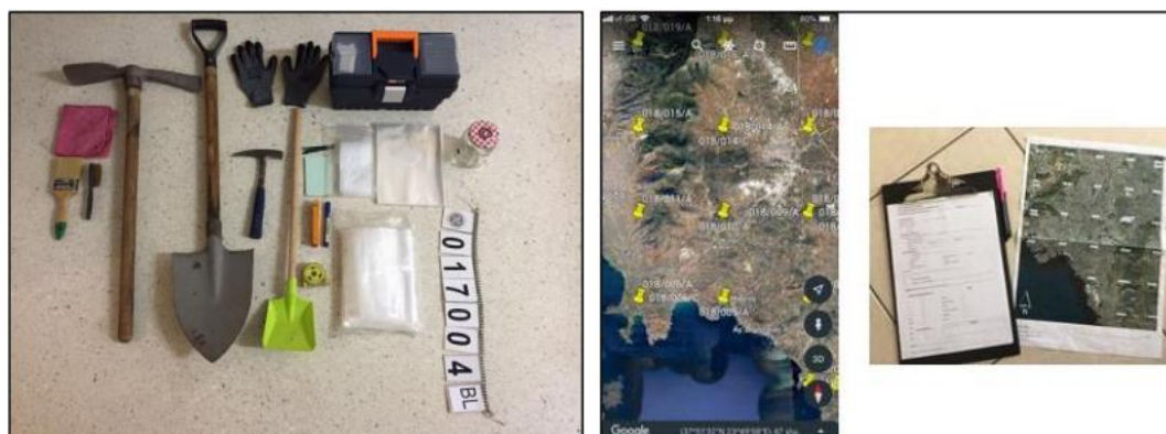
Figure 4. On the left: Sampling tools set for soil sampling. On the right: Print screen of a "smart" phone with the Google Earth application and the planned sampling locations, printed sampling form for field notes input, and a map of the sampling area with marked positions
