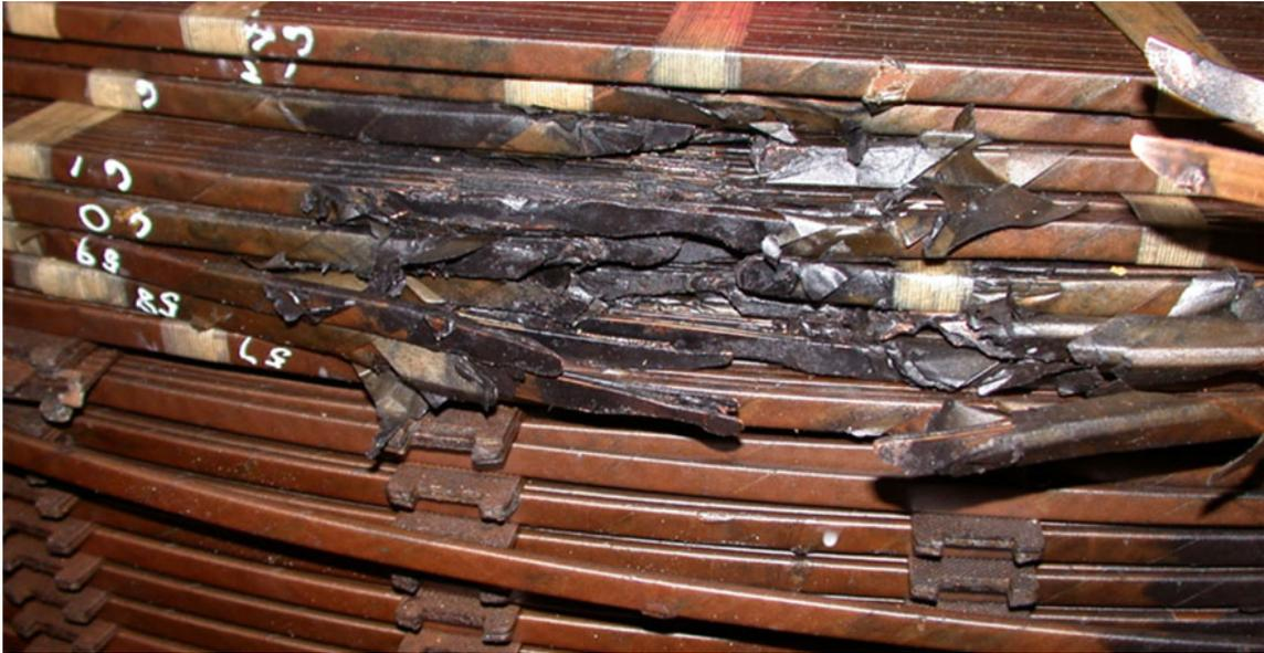
Figure 1.16: During the magnetic storm of Halloween 2003, GICs damaged the high voltage winding of this transformer at a large Eskom power station (South Africa), leading within a few weeks to a melted copper conductor and burned insulation, taking the transformer and associated 665 MW generator out of service. Credit: Trevor Gaunt, UCT. Source: <https://www.sansa.org.za>
