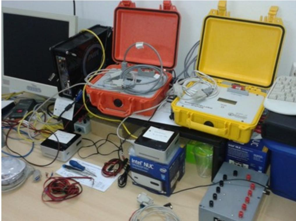
Figure 1.18: Photograph from DIO station instrumentation (GEOMAG-02M fluxgate magnetometer).
