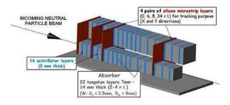
Figure 2.8: The LHCf Calorimeter
