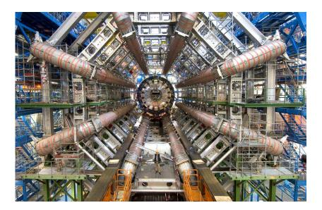
Figure 2.17: The ATLAS barrel Toroid
