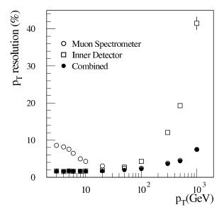
Figure 4.14:  $P_T$  resolution contributions on the combined muons
