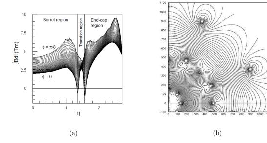
Figure 2.18: Torroid field details: Bending power  $\int Bd\ell$  vs.  $\eta$  (left), Field map in the transition region (right)
