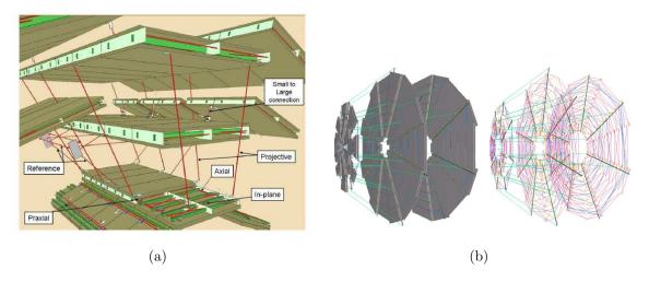
Figure 2.25: Principle of the alignment of the ATLAS muon spectrometer. Left: Barrel, Right: EndCups
