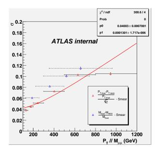
Figure 5.16: Comparison of  $\mathcal{P}_T$  and Mass resolutions vs.  $\mathcal{P}_T$
