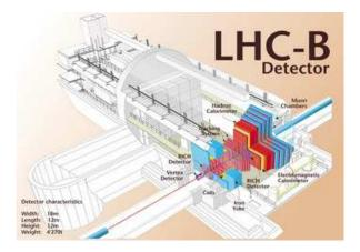
Figure 2.6: The LHCb detector
