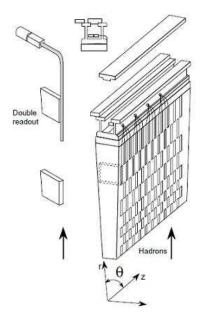
Figure 2.13: The principle design of ATLAS Tile Calorimeter
