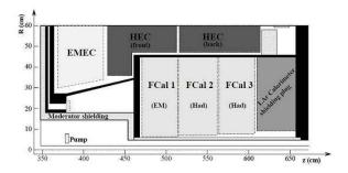
Figure 2.14: Schematic representation of the ATLAS Forward Calorimeter
