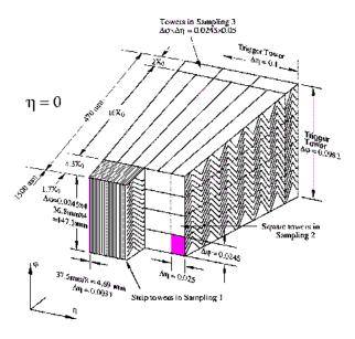
Figure 2.11: The accordion geometry of the ATLAS the Electromagnetic calorimeter
