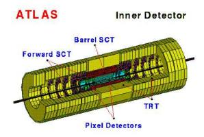
Figure 2.10: Schematic view of ATLAS Inner Detector
