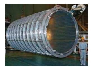
Figure 2.16: The ATLAS central Solenoid
