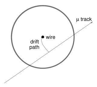
Figure 2.20: The MDT tube operation in a magnetic field
