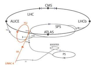
Figure 2.2: The LHC accelerating systems
