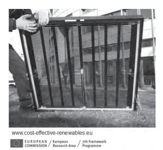
Figure 8: Prototype transparent solar thermal collector, developed in the European research project Cost-Effective. For details see chapter 7.6. Photo © Fraunhofer ISE
