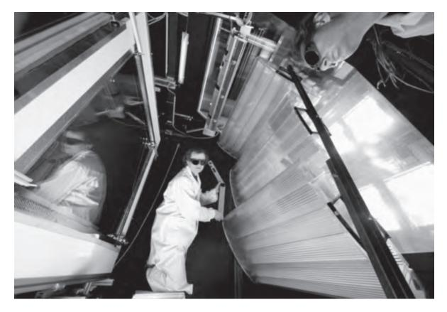
Figure 65: External blind consisting of large-scale slats, each with an ellipsoidal cover mounted for measurement in the calorimeter in the TestLab Solar Facades at the Fraunhofer Institute for Solar Energy Systems ISE in Freiburg, Germany. The slats have integrated translucent and opaque sections in order to enhance the daylighting and glare protection functionality. Pictures ©Fraunhofer ISE.
