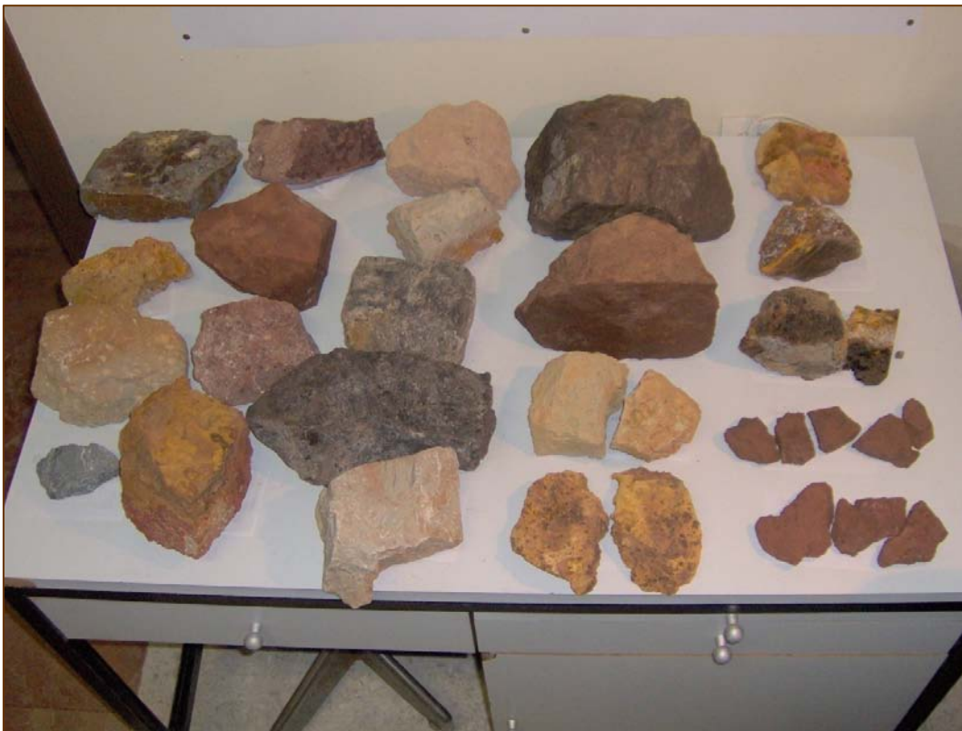
Figure 2.1.2: Bauxite (and limestone) samples in the laboratory before mineralogical and geochemical characterization.
