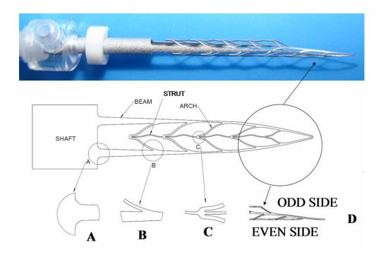
**Figure 1.** SAF file: Solid arrow shows beam, hollow arrows show arches and dashed arrows show struts. Figure 1b shows the connecting points of the components: (A) beam to the shaft, (B) arch to the beam and (C) strut to the arch.
