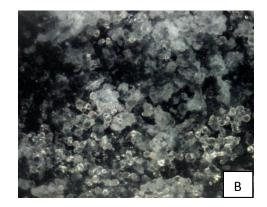
Figure 7 Sodium chloride (NaCl) crystals at A. 200x and B. 500x magnification
