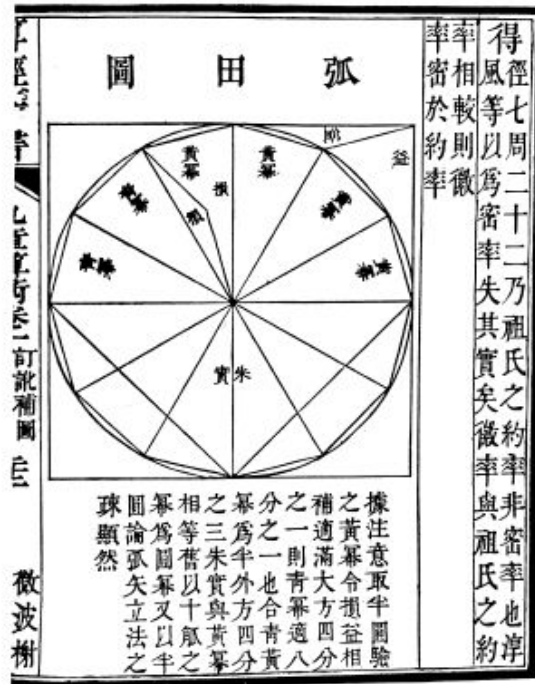
Fig. 8. Slicing \pi more finely: one of Dai Zhen's illustrations for the 九章算術 ( Jiu Zhang Suan Shu, The Nine Chapters on the Art of Mathematics ), where Liu Hui's method of approximating the value of \pi by inscribing regular polygons is demonstrated.
