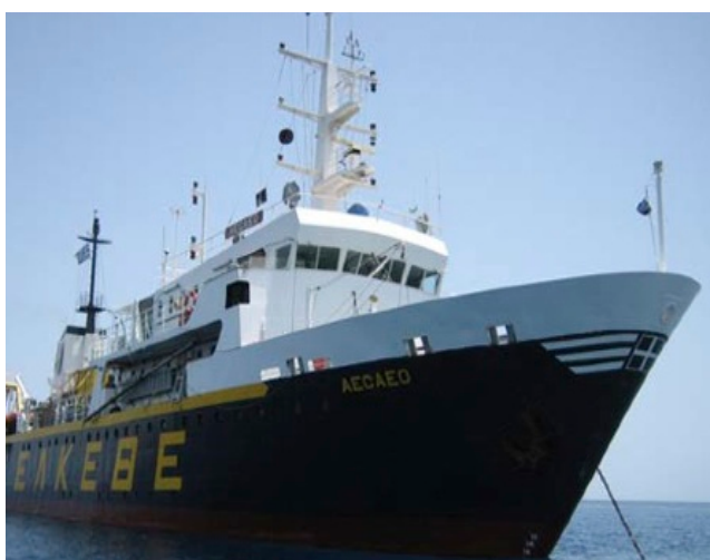
Figure 4.3 Research Vessel AEGAE0 (HCMR), 62.00m in length, may reach 12.50 knots maximum speed.
