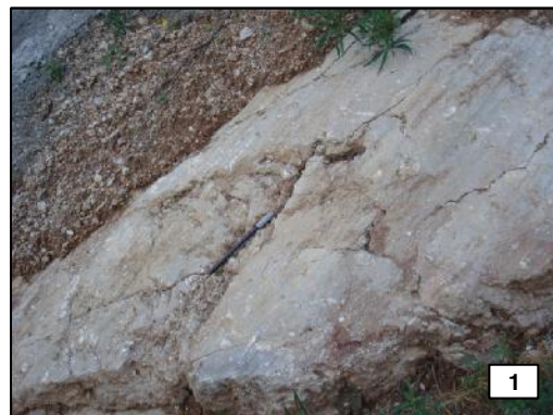
Figure 1 : Reveiled part of the Psathopyrgos fault plane towards Panagopoula. Dip & dip direction of the fault plane: 41° / 348° & 41° / 355°.
