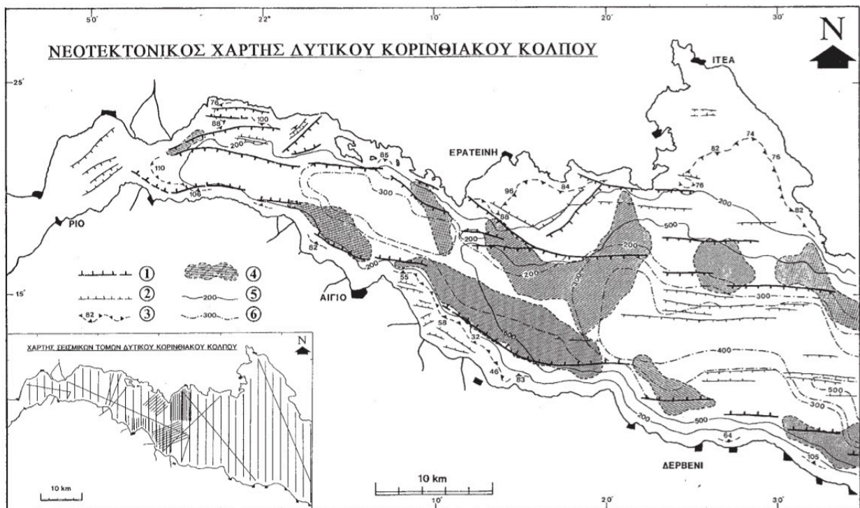
Figure 3.4 Neotectonic framework of the Corinth basin. 1: Major active faults, 2: Secondary active faults, 3: Continental platform boundary, 4: Active submarine landslides areas, 5: Isobaths (offshore) 6: Contour lines (onshore) – after Papanikolaou et al, 1997 .
