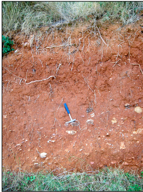
Figure 5.1 Alluvial deposits consisting of clays with angular fragments of Pindos limestones.
