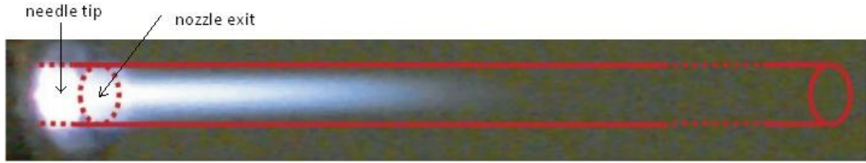
Figure 3.2: The cylinder representation of the plasma jet device [30].
