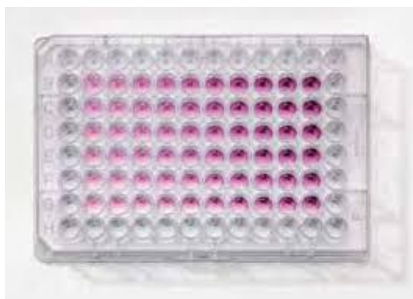
Figure A.3. The different nuances obtained after the MTT assay in a 96-well plate. More intense color signifies a higher number of viable cells [11].
