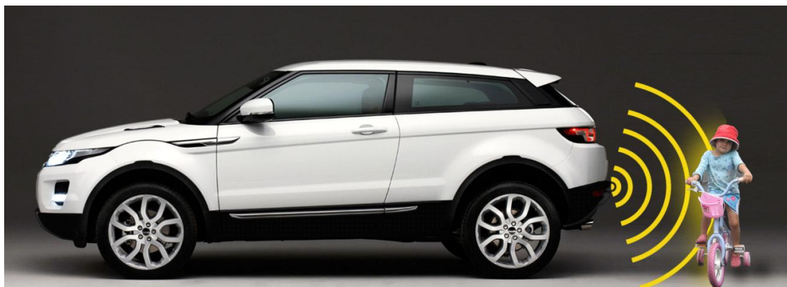
Parking sensors detect objects behind the car and beep to alert the driver
