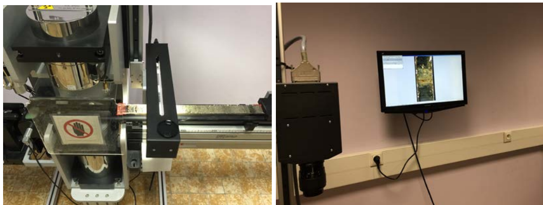
Figure 25: Scanning of the cores and recording of magnetic susceptibility at the CNRS laboratory, at Bensaçon, France.
