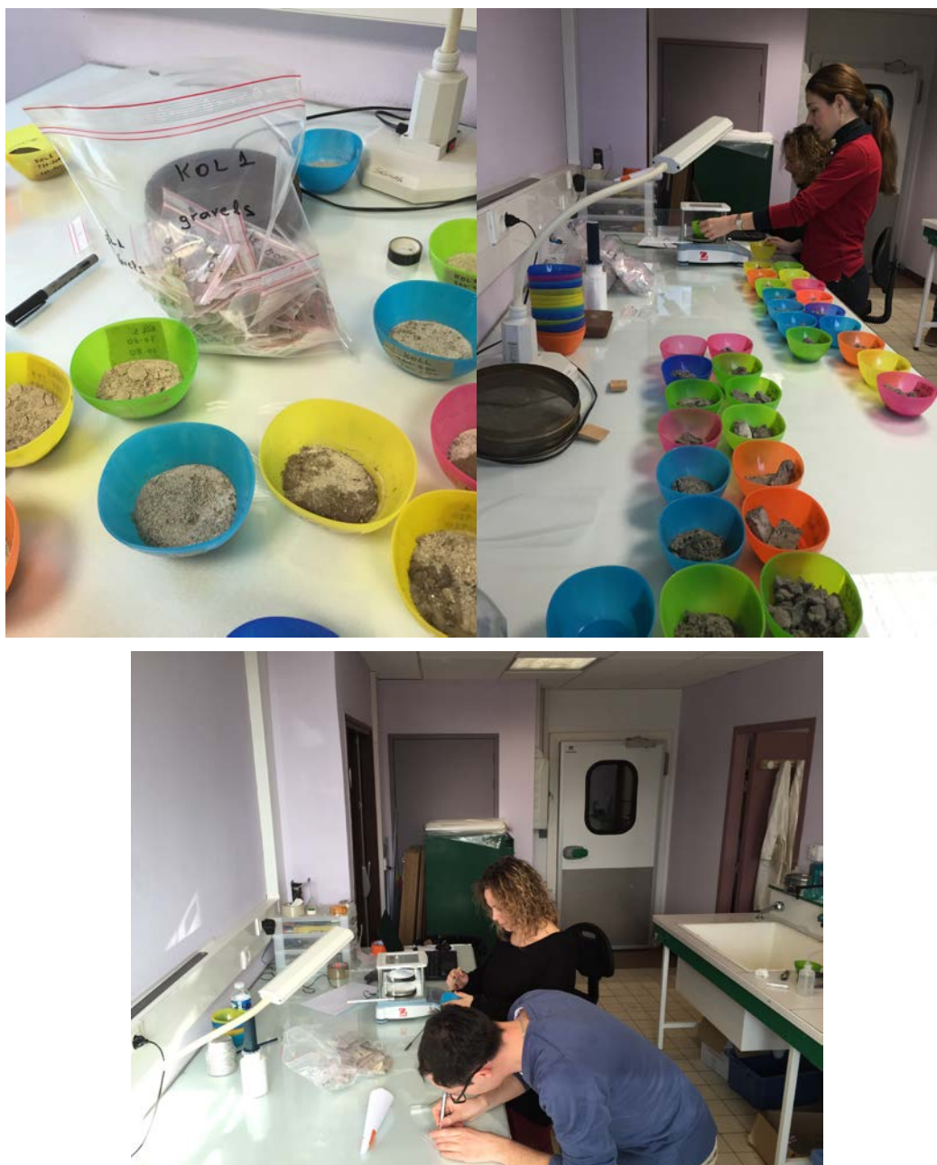
Figure 26: Each core was divided into sub-samples, which were oven-dried, weighted and separated through sieving to gravels, sands and silts-clays.
