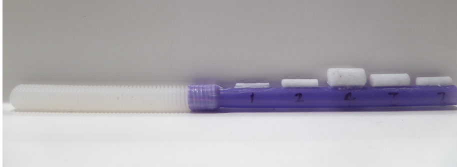
Figure 6.9: The final set of calcium lesion phantoms. From left to right: 240\text{mgCaCO}_3/\text{cm}^3 1 mm, 200\text{mgCaCO}_3/\text{cm}^3 2 mm, 160\text{mgCaCO}_3/\text{cm}^3 4 mm, 160\text{mgCaCO}_3/\text{cm}^3 3 mm, 160\text{mgCaCO}_3/\text{cm}^3 2 mm. All calcium lesion phantoms have a length of 8 mm.
