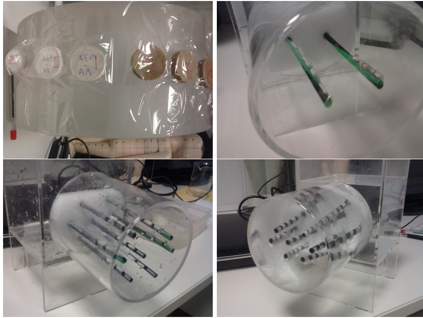
Figure 6.4: Measurement setups of different materials in different stages of the calcium phantom construction. top left: Various different materials taped on a Plexiglas phantom. top right: The first set of small lesion equivalents in small sizes glued onto small plastic sticks. bottom: The final lesion equivalent measurements before the end selection.
